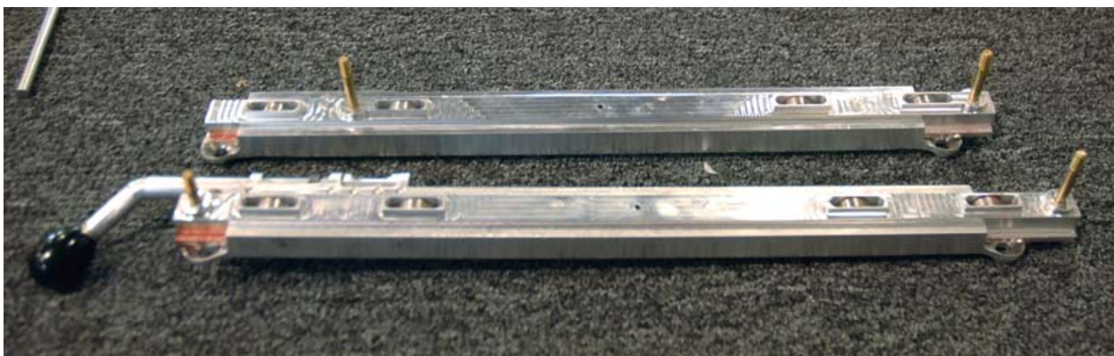
We made custom billet seat rails. They ride on four bearings each.
