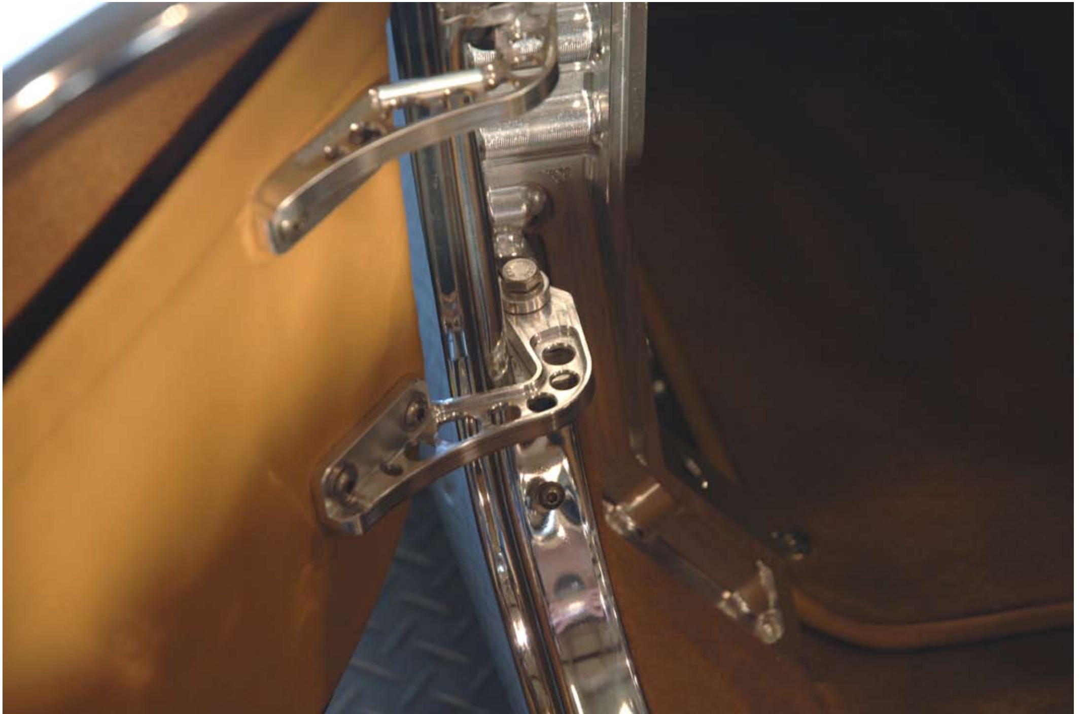
The door hinges were hollowed out to save as much weight as possible. They pivot on stainless pins.
