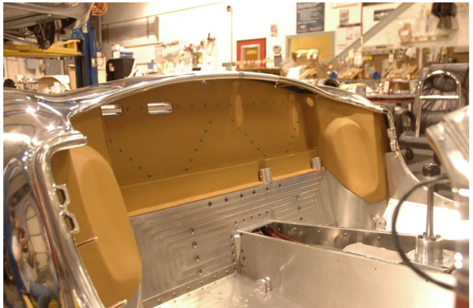
We used stainless button-head screws in the rear bulkhead on top of the leather as a nod to the billet chassis. Notice the holes for the passenger shoulder harness in the top, right side of the rear bulkhead (left side in the picture). All the bolts in the interior were either button heads or counter sunk for a flush fit.
