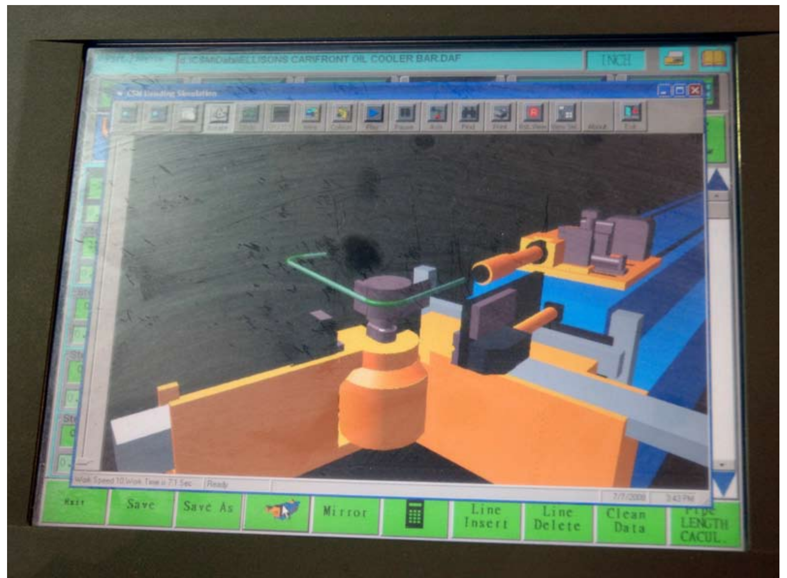
The CNC tube bender allows the operator to program the tube and virtually bend the part to make sure nothing crashes.
