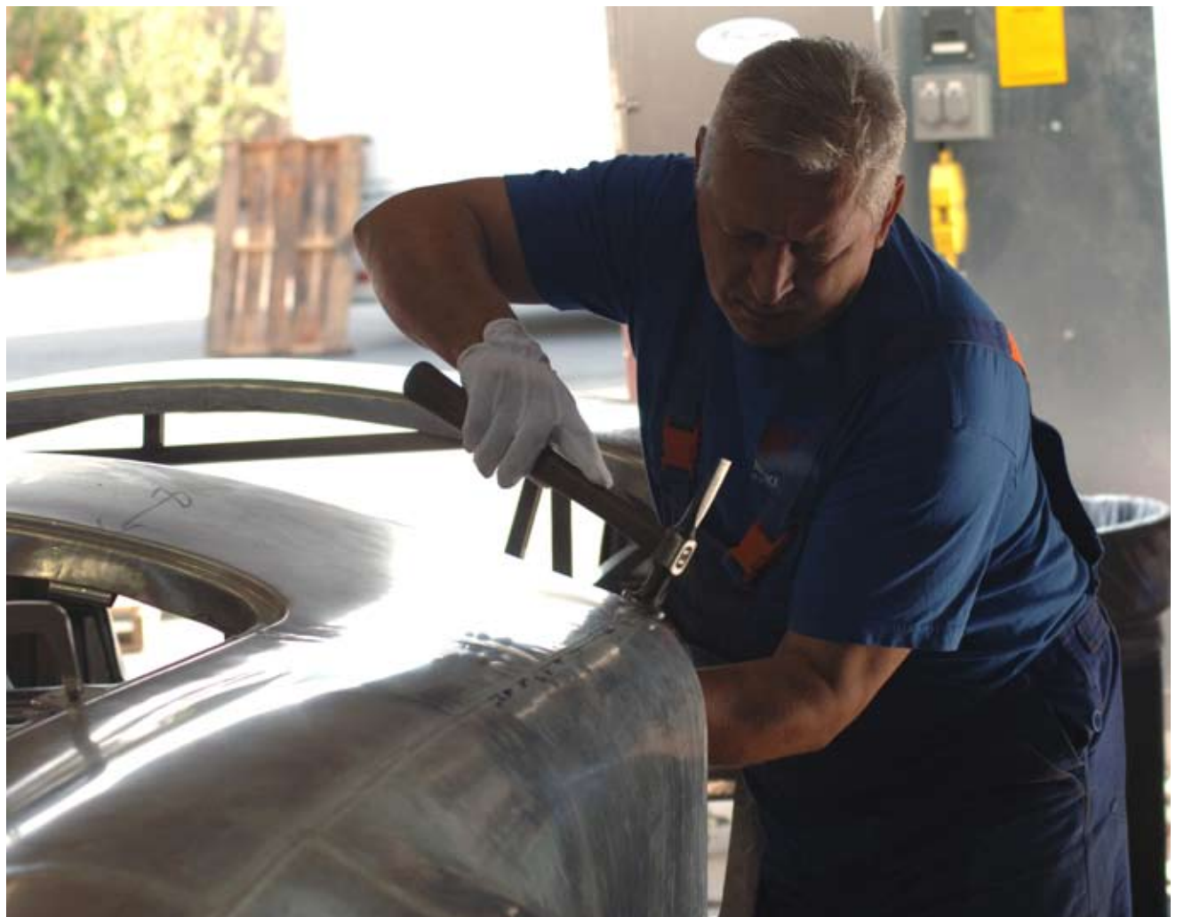
He then rubs his hand over the surface of the metal. An experienced craftsman can tell the subtle differences between high spots and low spots. A hammer is typically used to do the gross straightening of the panel. His left hand is holding a “dolly” or a heavy piece of metal that generally conforms to the shape of the panel to back up the hammer blows and help straighten the metal.
