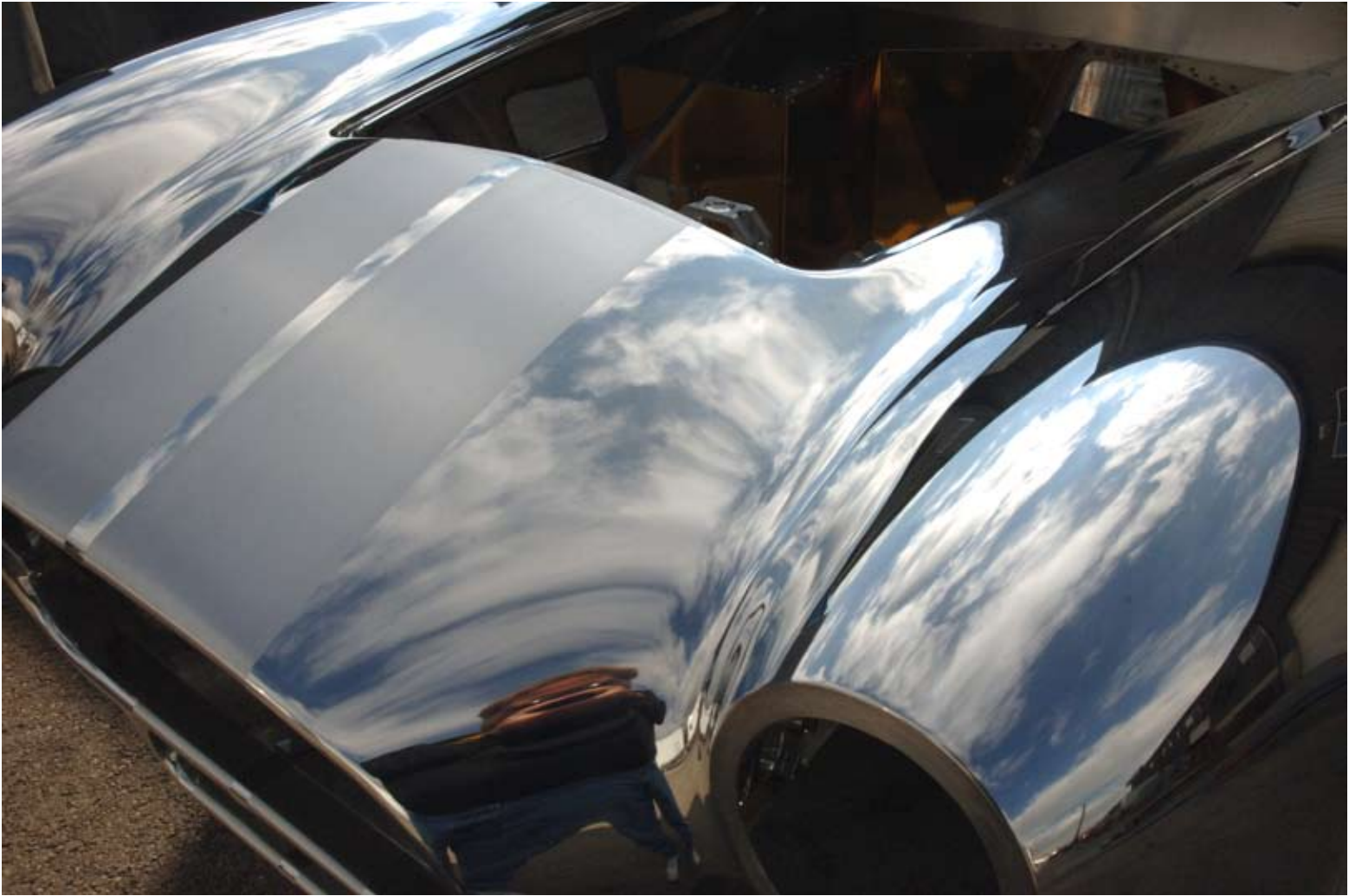
Final polishing and striping on the body. The car is completely polished first. Then, the stripes are laid out on the body and sanded into the polished finish with 220 grit sand paper.
