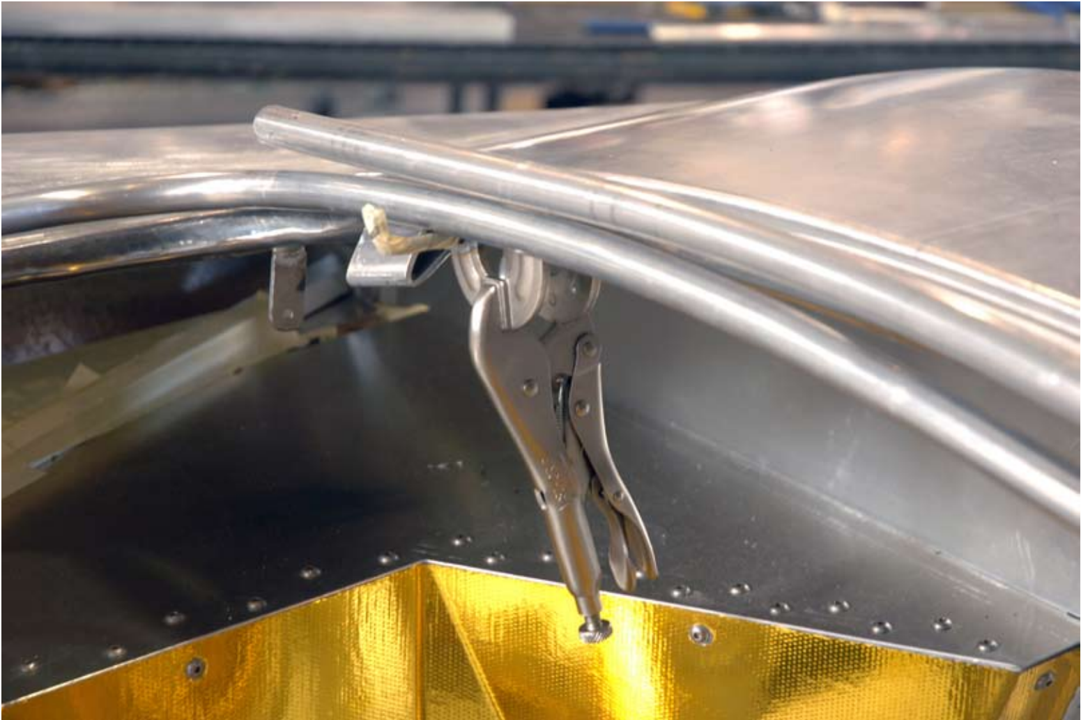
To support the rear of the hood in the right place, we drilled and tapped a hook into some Vise-Grip pliers then placed the tubes on the pliers. The hood tubes were then cut to length and welded together.
