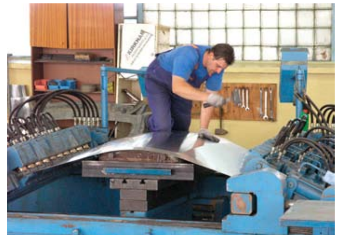
Using a rubber mallet to define the edges of the hood.
