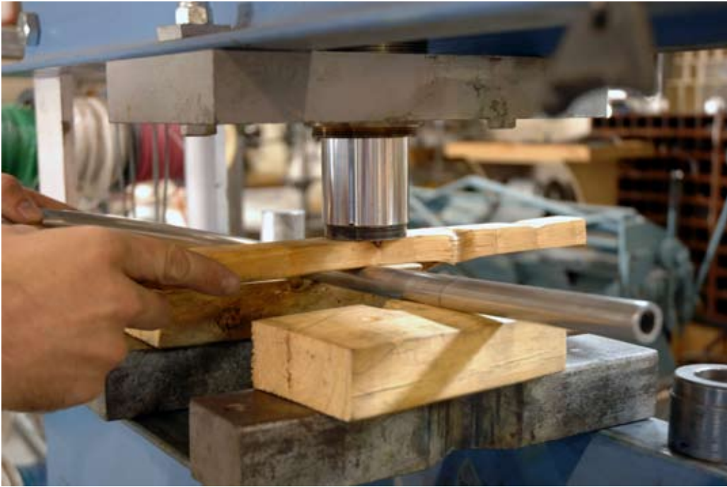
As we built the substructure tubes, any tube that needed a little tweaking was bent in the press between blocks of wood.
