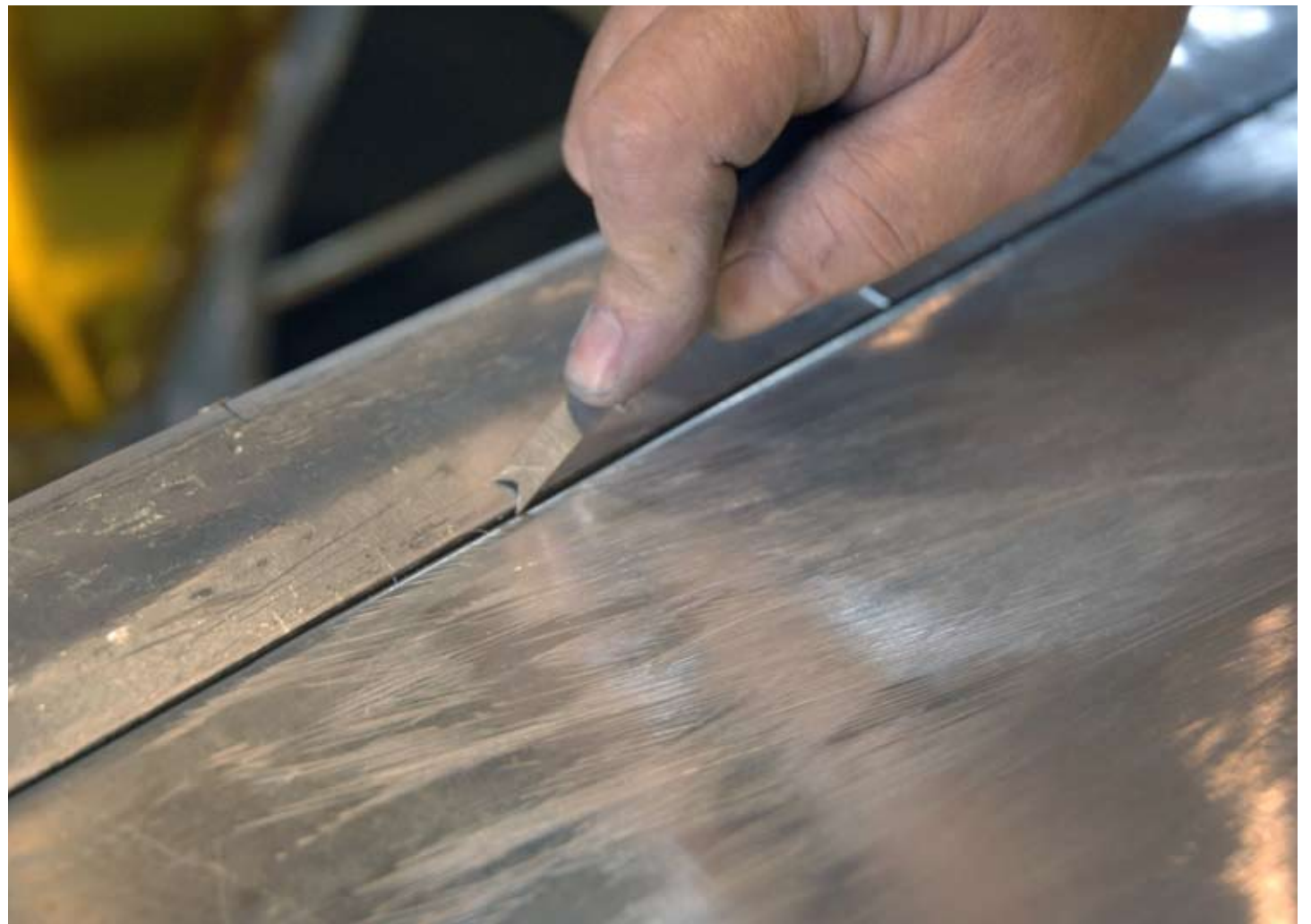
A custom scribe marks a line into the hood flange. One leg of the scribe is longer than the other so it can easily ride against the hood jam. The distance of the scribed line is \frac{3}{16} of an inch for the desired gap plus \frac{1}{16} of an inch for the thickness of the hood skin.
