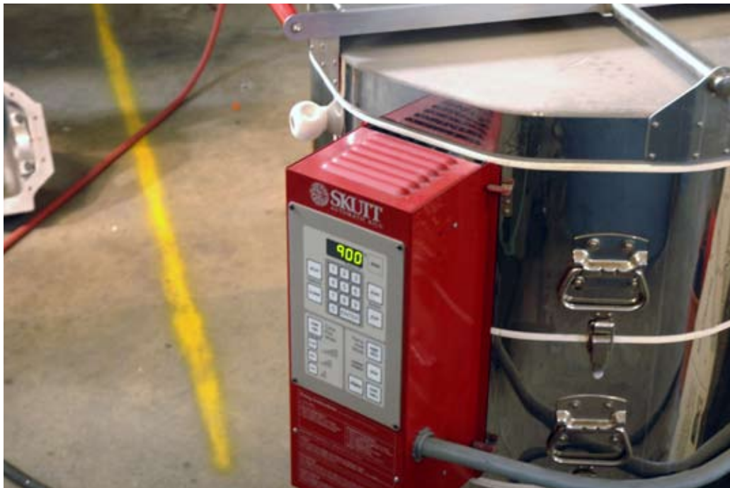
All of our 17-4 parts are heat treated in an oven we specially modified with high-accuracy thermocouples.
