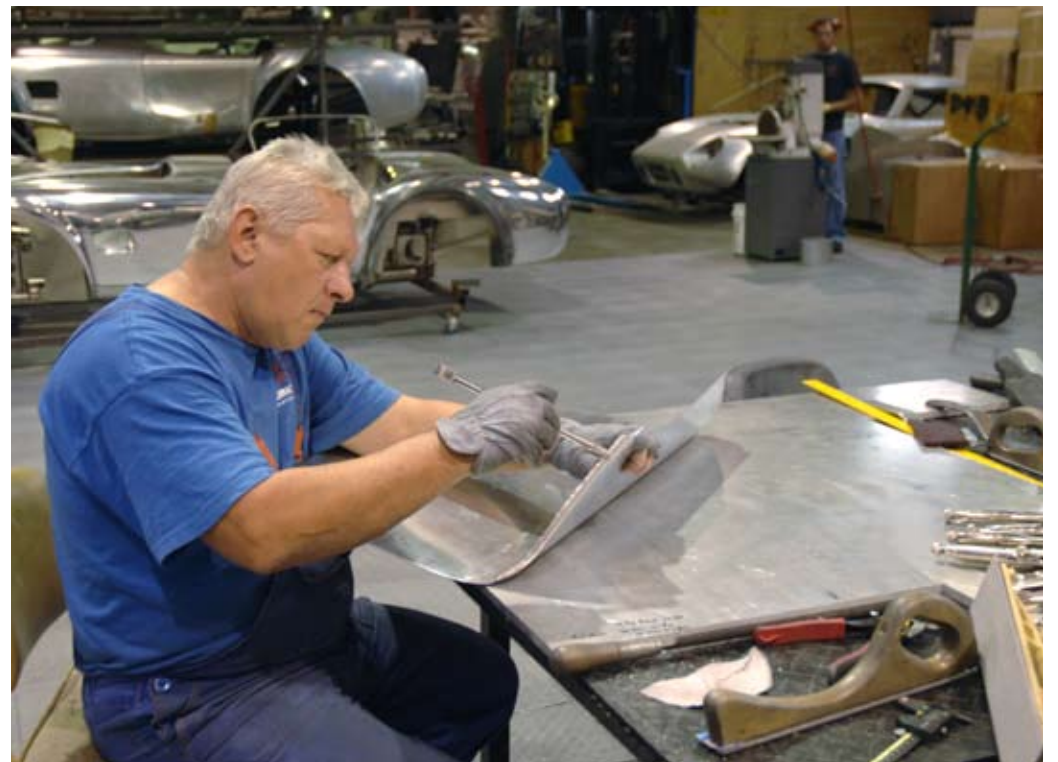
Bending the 90 degree hem into the door skin.
