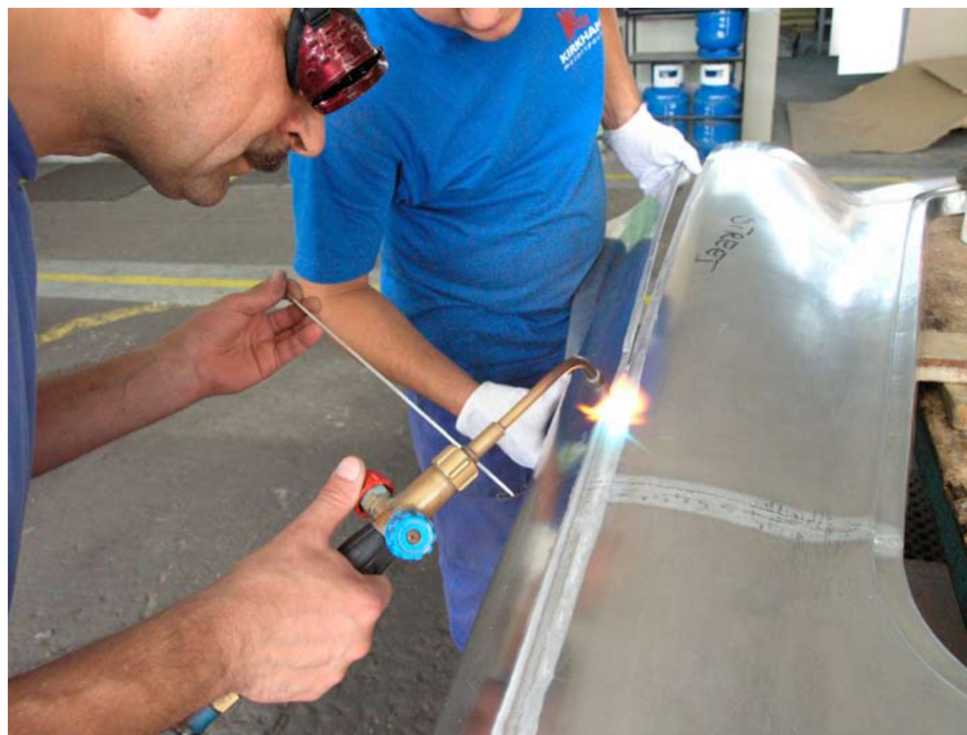
The panels are then trimmed and welded together with an oxyacetylene torch. We gas weld panels together for a number of reasons. Gas welding is much faster than TIG welding. Gas welding leaves the metal very soft and malleable, whereas TIG welding tends to make brittle welds. Finally, gas welding leaves a very flat bead that is easy to completely erase with a file. Photo by Kirkham Motorsports Poland.
