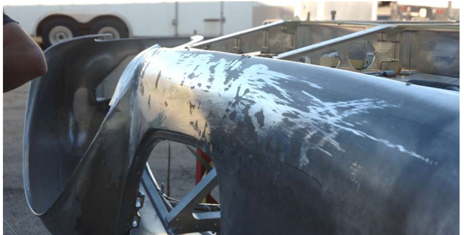
The rockers were “pick and filed” smooth once they were riveted down.
