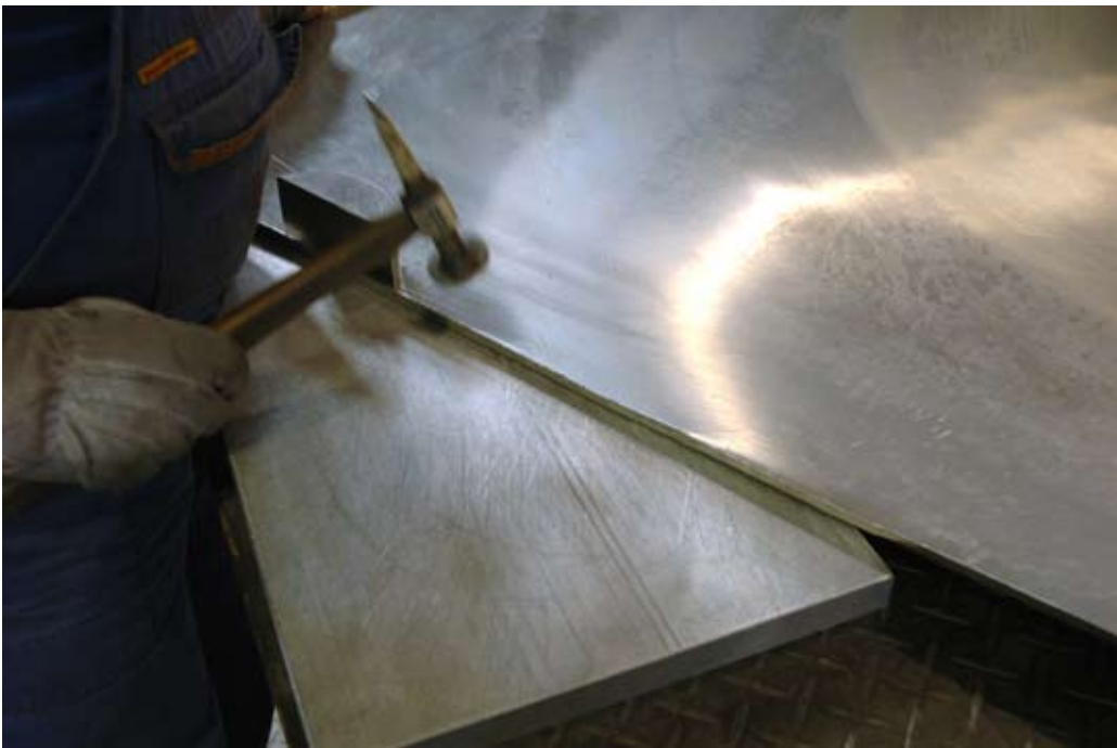
Once the hem is straightened out, we take a hammer and strike the edge of the hem to tighten up the radius.
