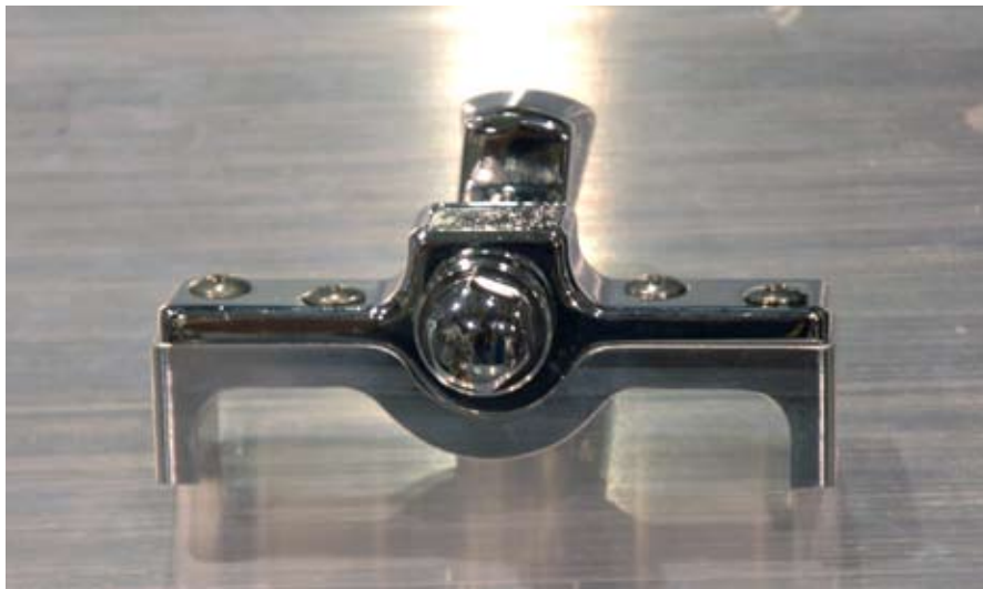
The door striker was bolted to a billet striker bracket and then tack welded to the frame.
