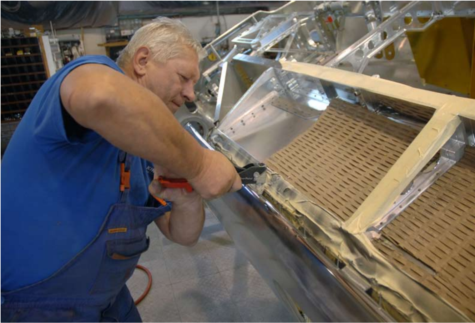
Once the rockers were wrapped, they were riveted to the body tube.
