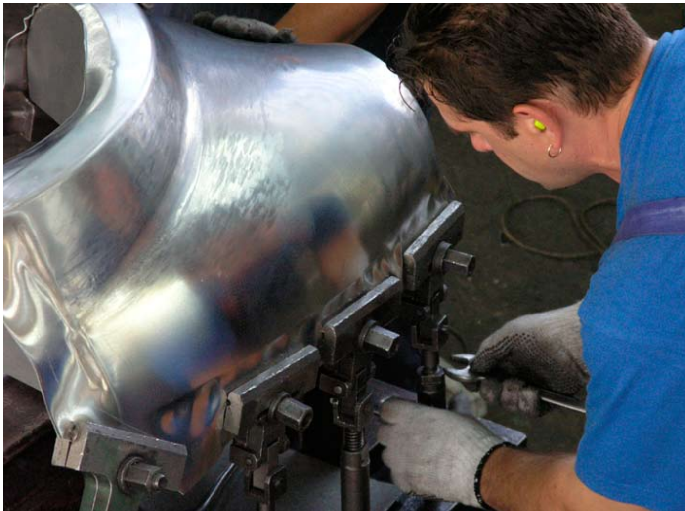
The holding clamps are tightened as the aluminum is shaped. Photo by Kirkham Motorsports Poland.
