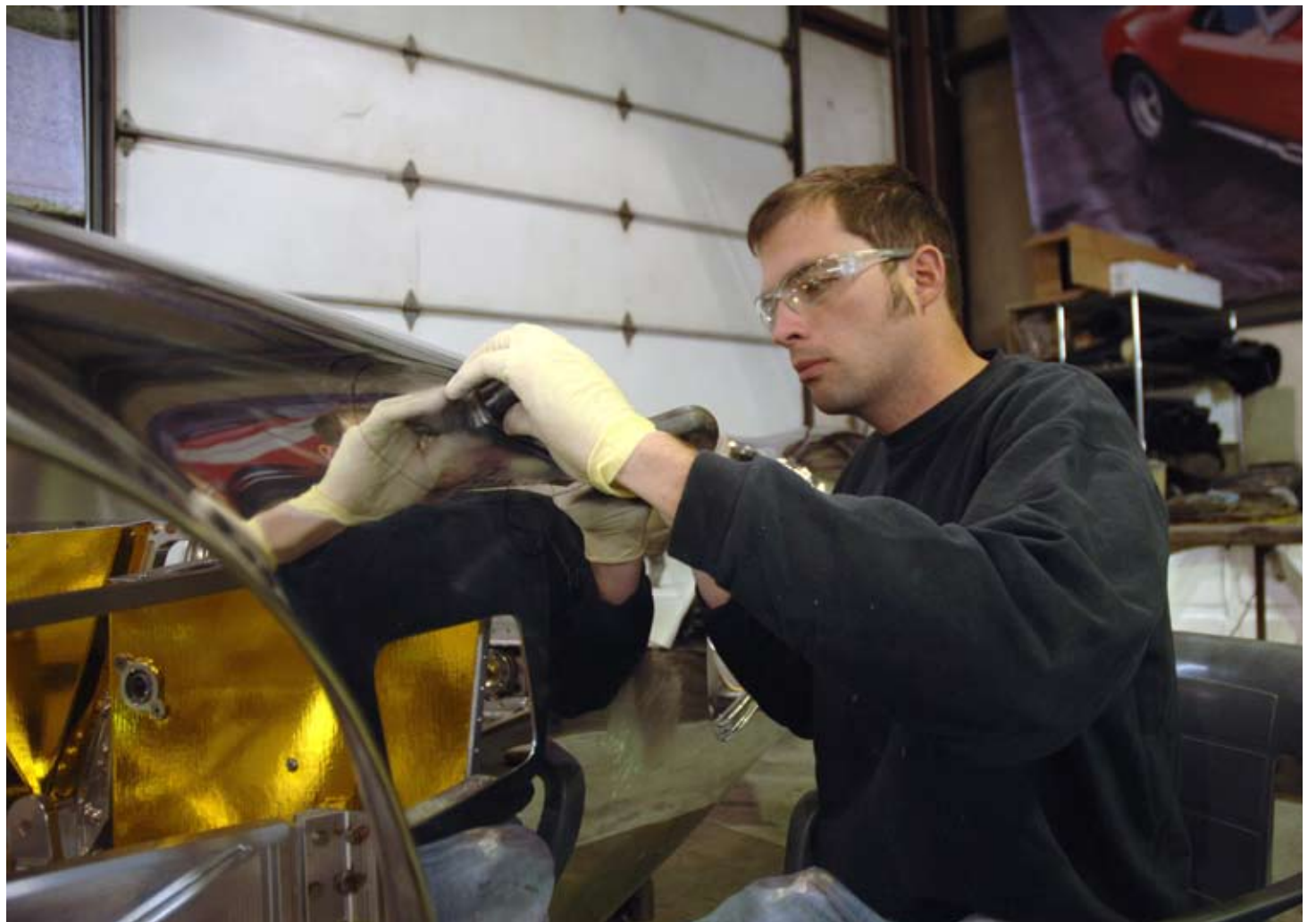
Right: Sandwich found a few waves even after the body was polished.
