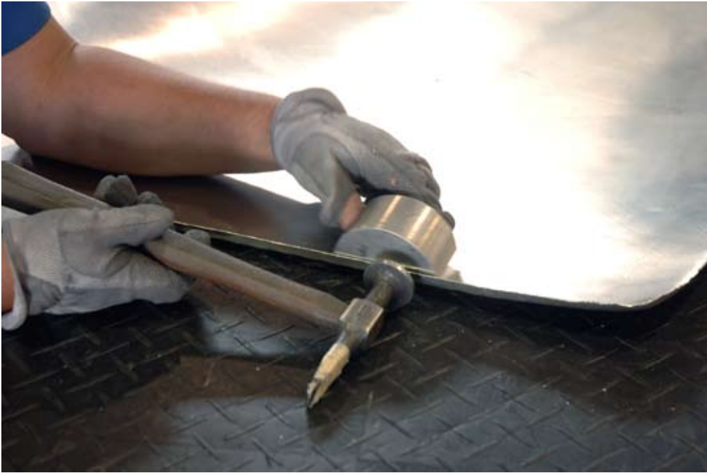
Next the hem is flattened with a hammer and dolly.
