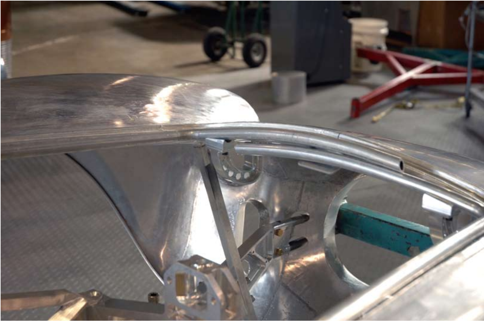
The hood hinges need to be mounted to get the hood tubing in the right place.
