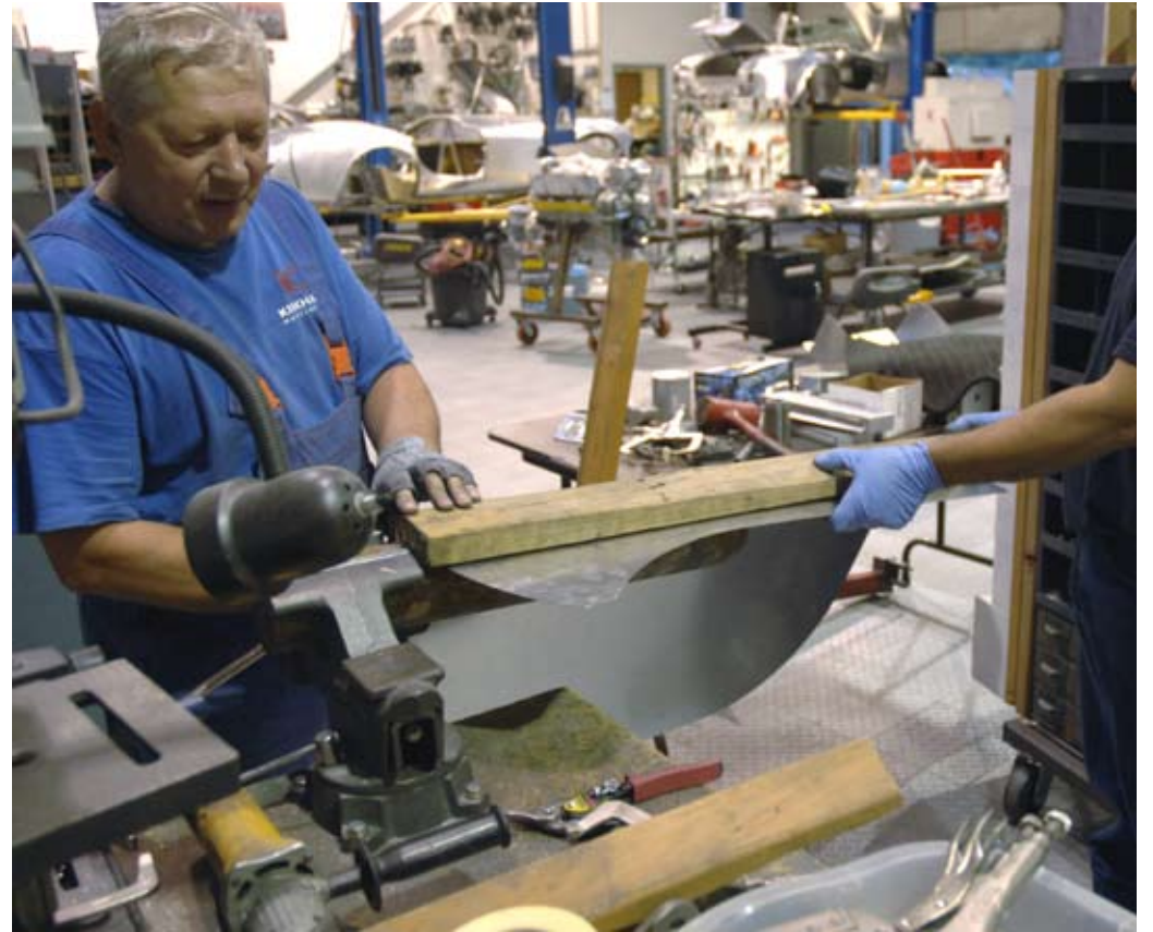
The large curve of the door is made by bending a sheet of aluminum over a 4-inch pipe.
