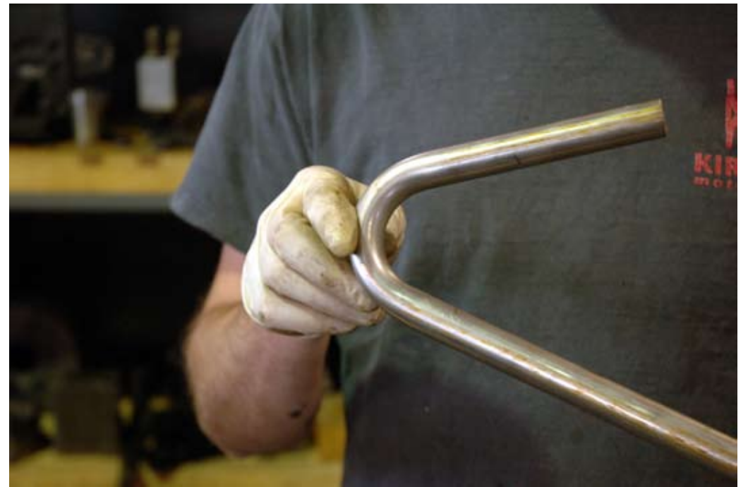
The clamps had to be made to very tight tolerances because we were bending heat-treated 6061 T6 tubing without annealing it. We had to buy a special, drawn tube for the bends we wanted.
