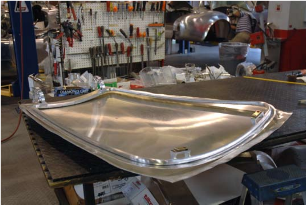
The hood frame is placed on the upside down hood skin and adjusted to fit.
