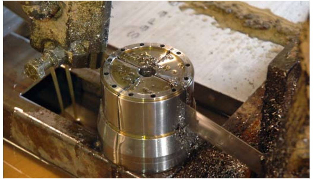
We made the “C” axis clamping collet for the push bender.
