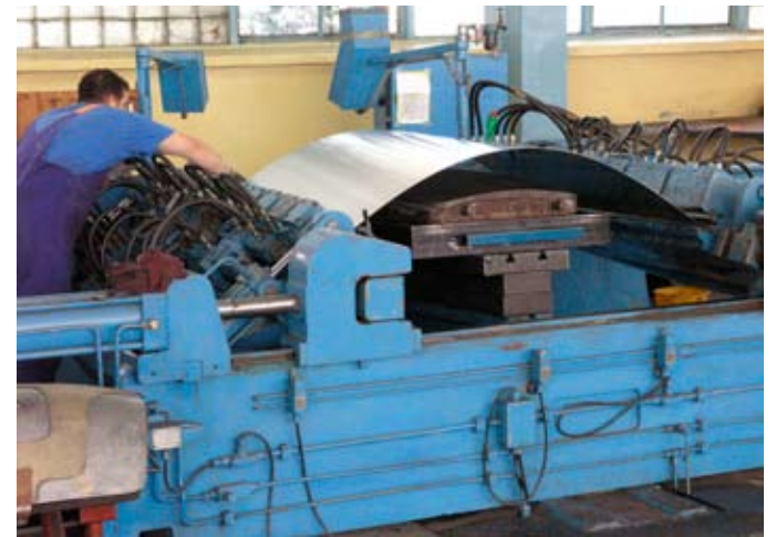
Aligning the jaws to grab the aluminum sheet uniformly on both sides.
