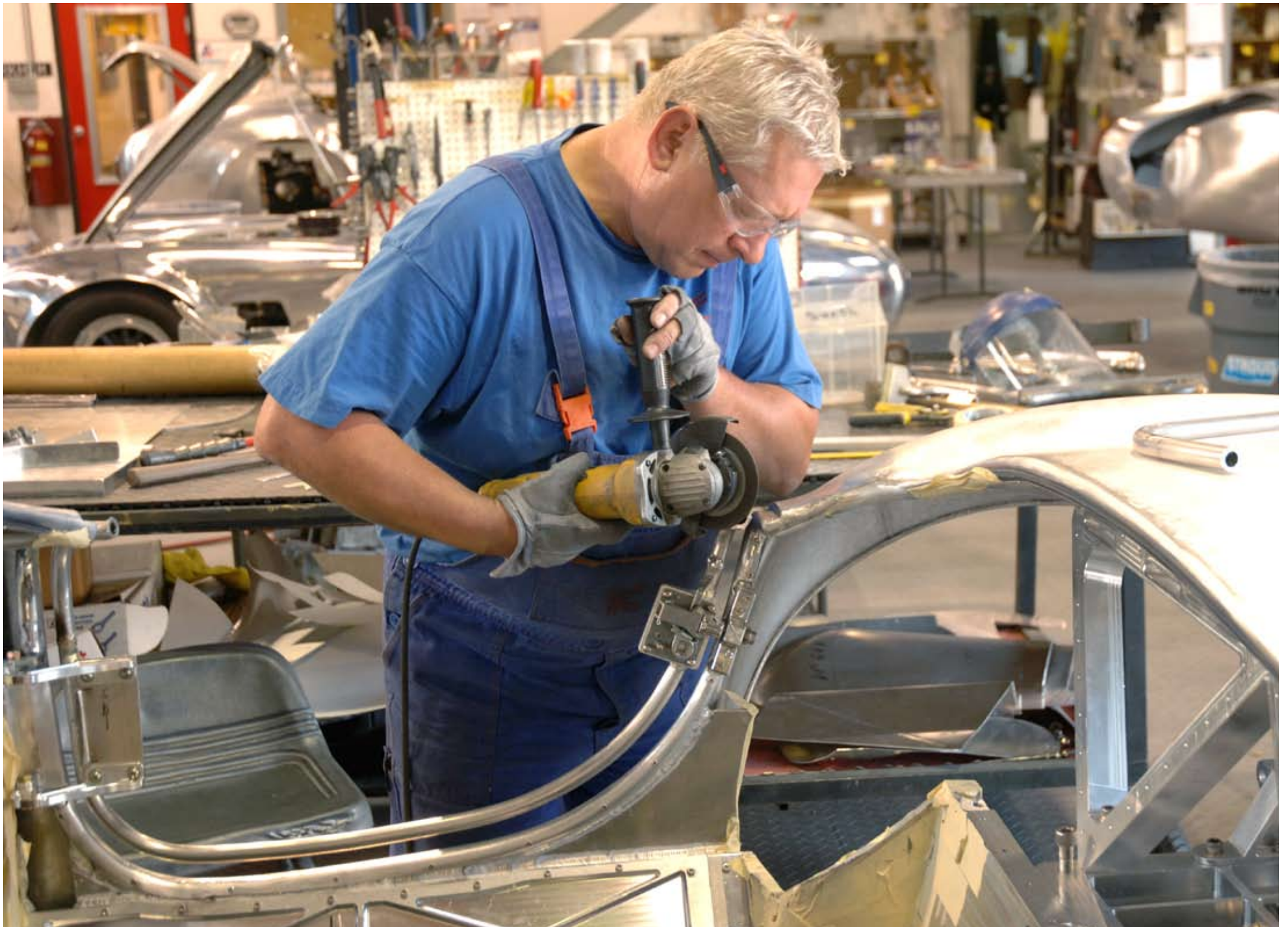
Beginning work on the door frame tubes. The hinge, striker, and latch are functional at all times to make sure the door works.
