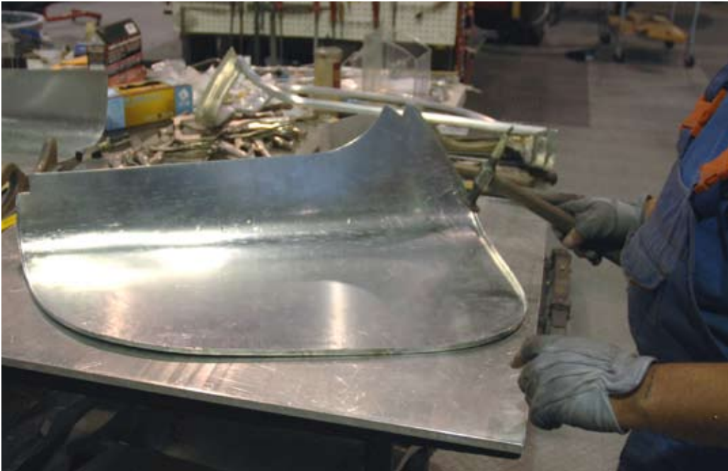
Squaring up the radius. We work on a flat sheet of aluminum to keep everything as square and flat as possible.
