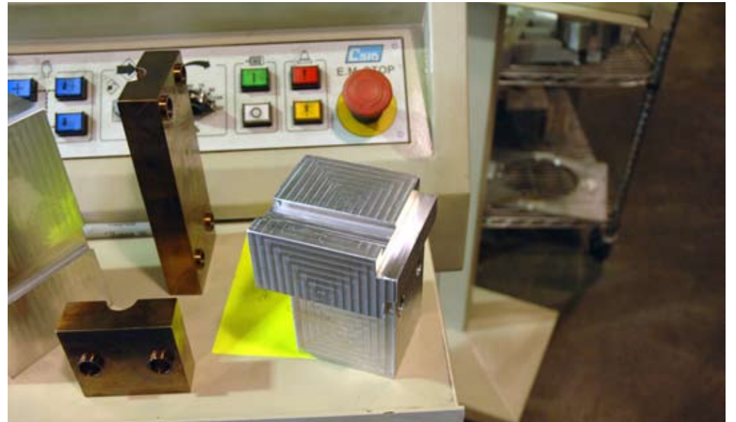
Custom clamp tooling for the 3/4 inch substructure. The working dies were made from 17-4 PH stainless steel.
