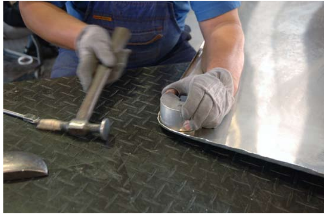
The half moon dolly is shaped to fit into the radius of the hood skin.
