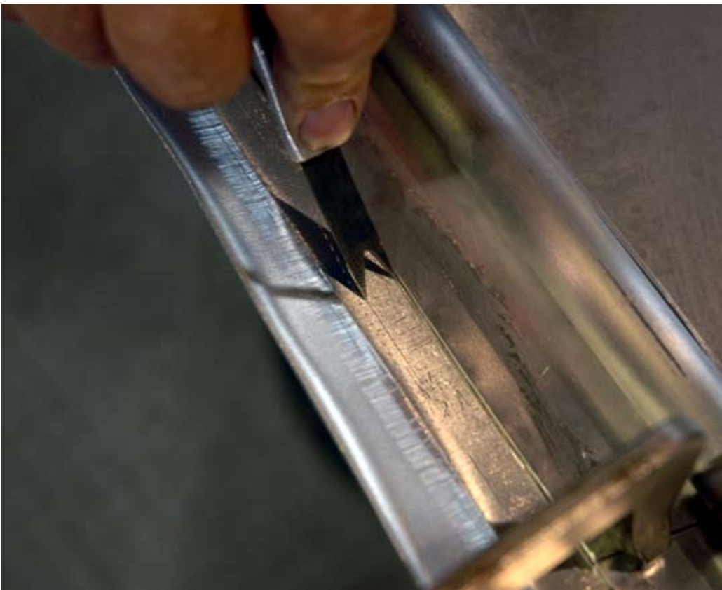
Marking the distance of the hem with a tool similar to the flange scribe.
