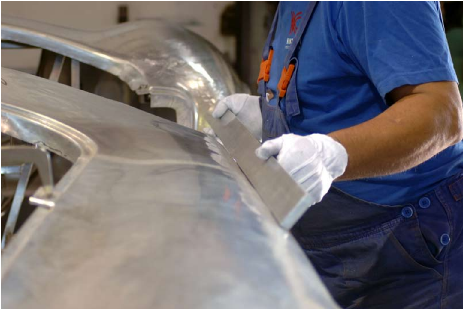
Jozef places a straight edge on a panel to check it for straightness. Light shows under the edges where the panel is not straight.
