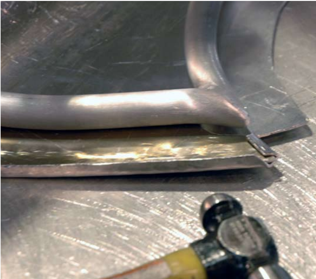
Once the door frame is in the door skin, a small tab at the front and rear of the door is bent over to lock the skin into place. Then, the rest of the door can be easily hemmed.
