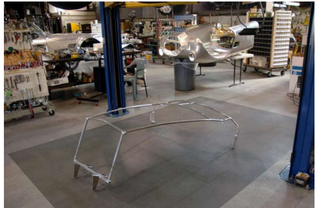
The front substructure cage after welding.
