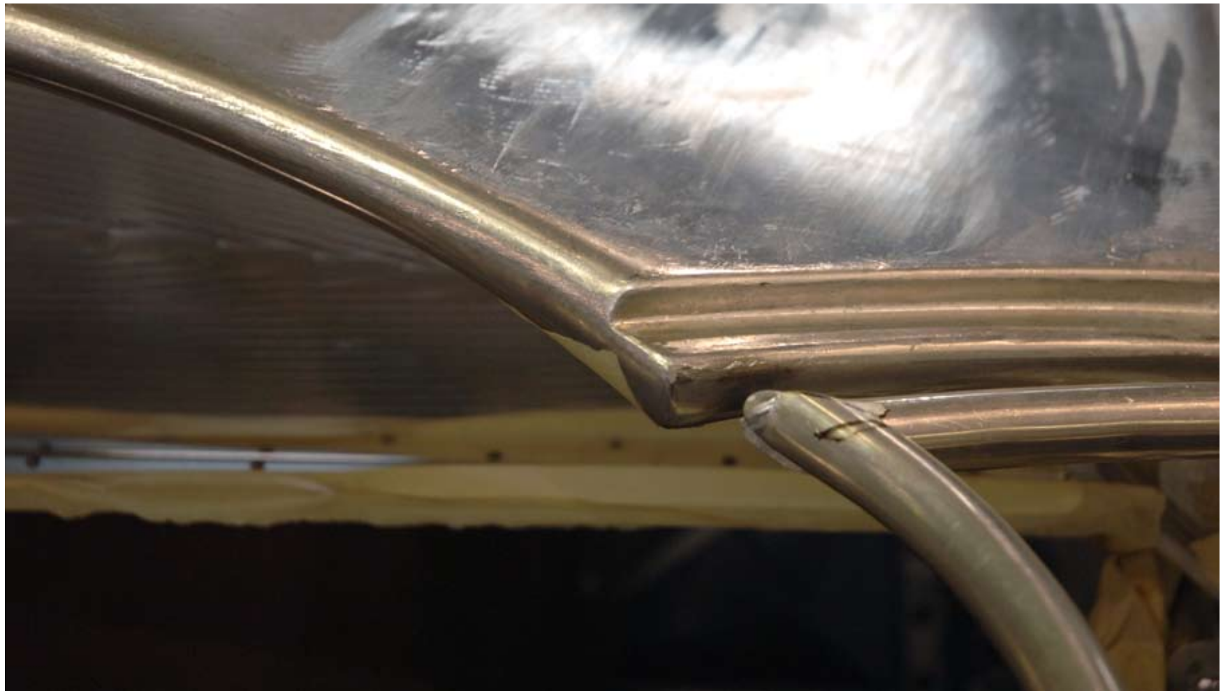
The door frame sweeps have to line up perfectly with the body.
