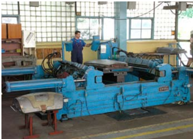
Making a hood on a stretch press is much like stretching cellophane over a container of food.
