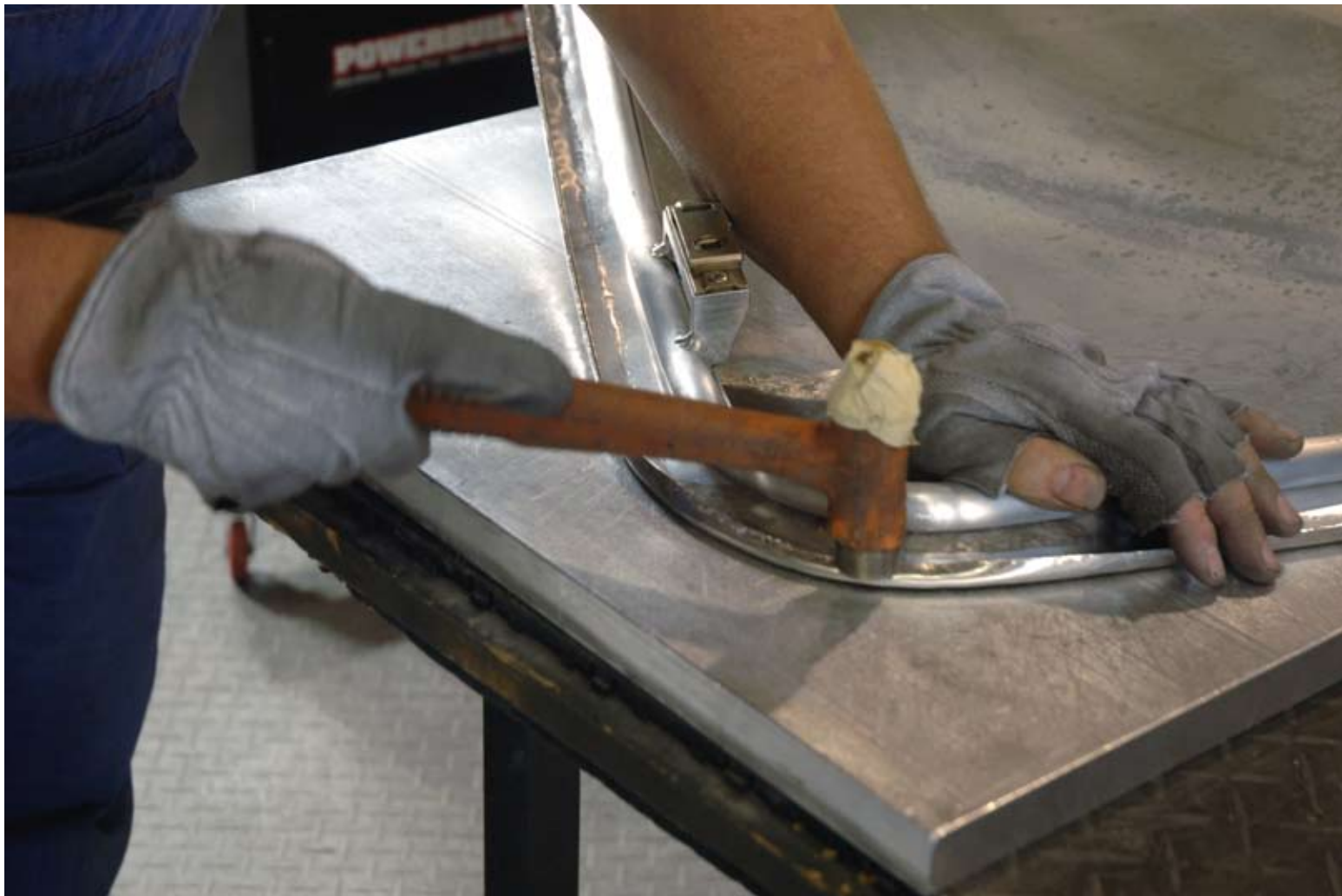
A steel hammer is used to close the hem 180 degrees and to fold it flat.
