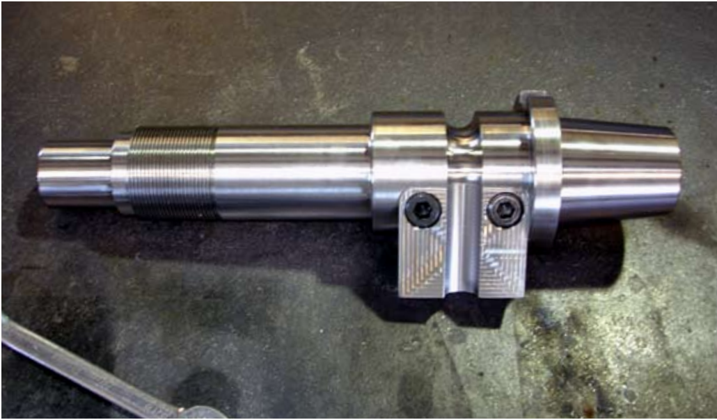
We cut the required 3/4 inch substructure radius right into our custom-made axle. We then machined a pocket in the axle for the clamp die.
