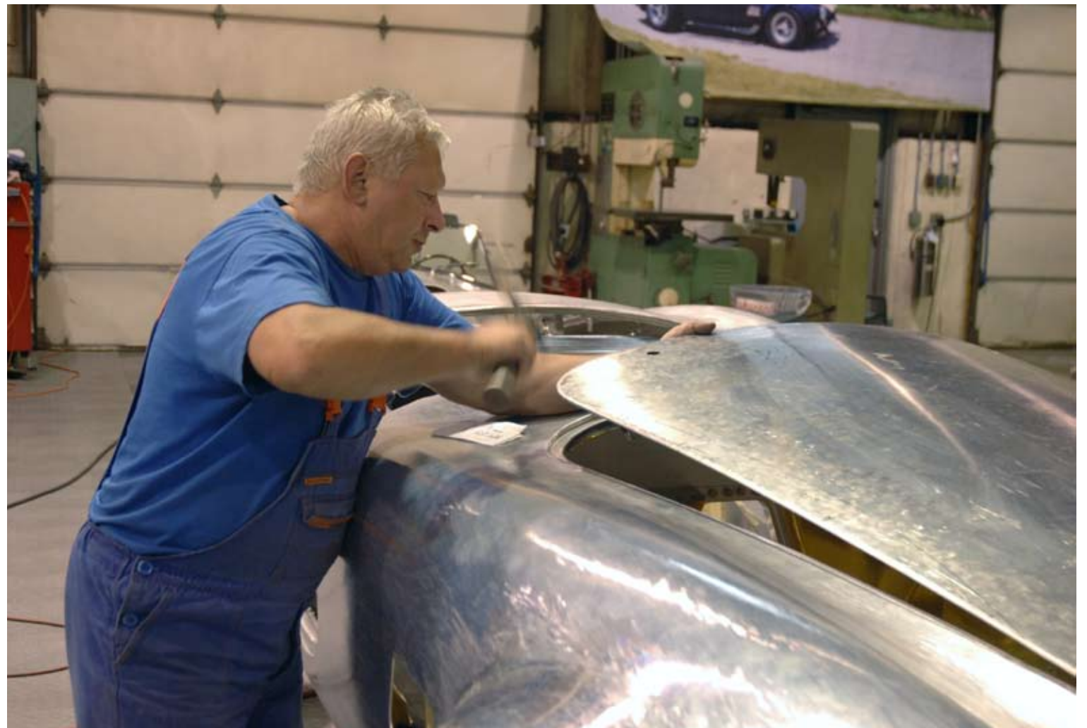
With a steel hammer, we move the hood lines until they fit just right.
