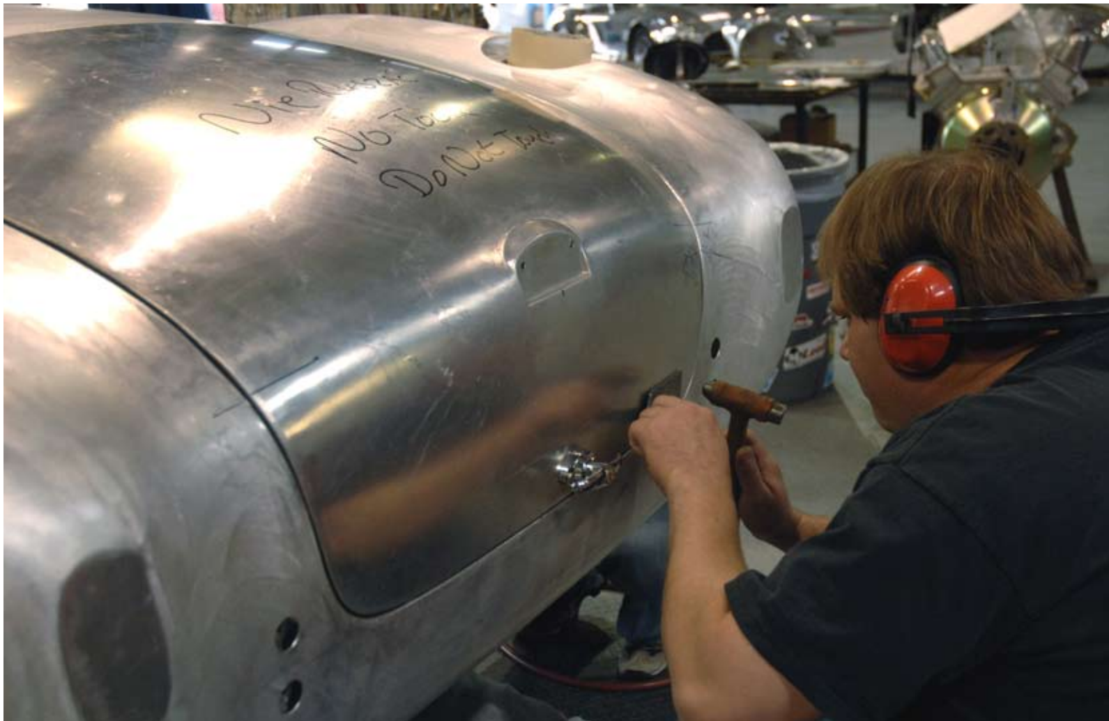
Here I am tapping on a slapper with a hammer, spreading the blows out to do the final tuning of the trunk lines.
