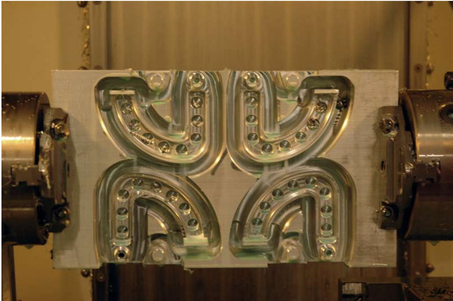
The hood and trunk hinges are identical; we machined them from the same plate.
