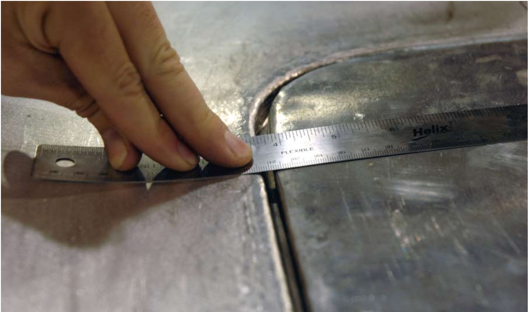
After hammering them with a special dolly, we were able to square up the jams quite nicely. Again, the steel rule lies flat across the jam.
