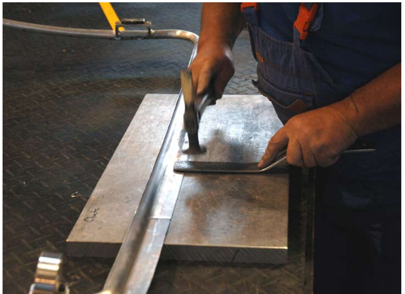
Straightening the hood flange with a hammer tapping on a slapper. The hinges and hood latches are mounted to the frame to make sure the hood opens and closes properly.
