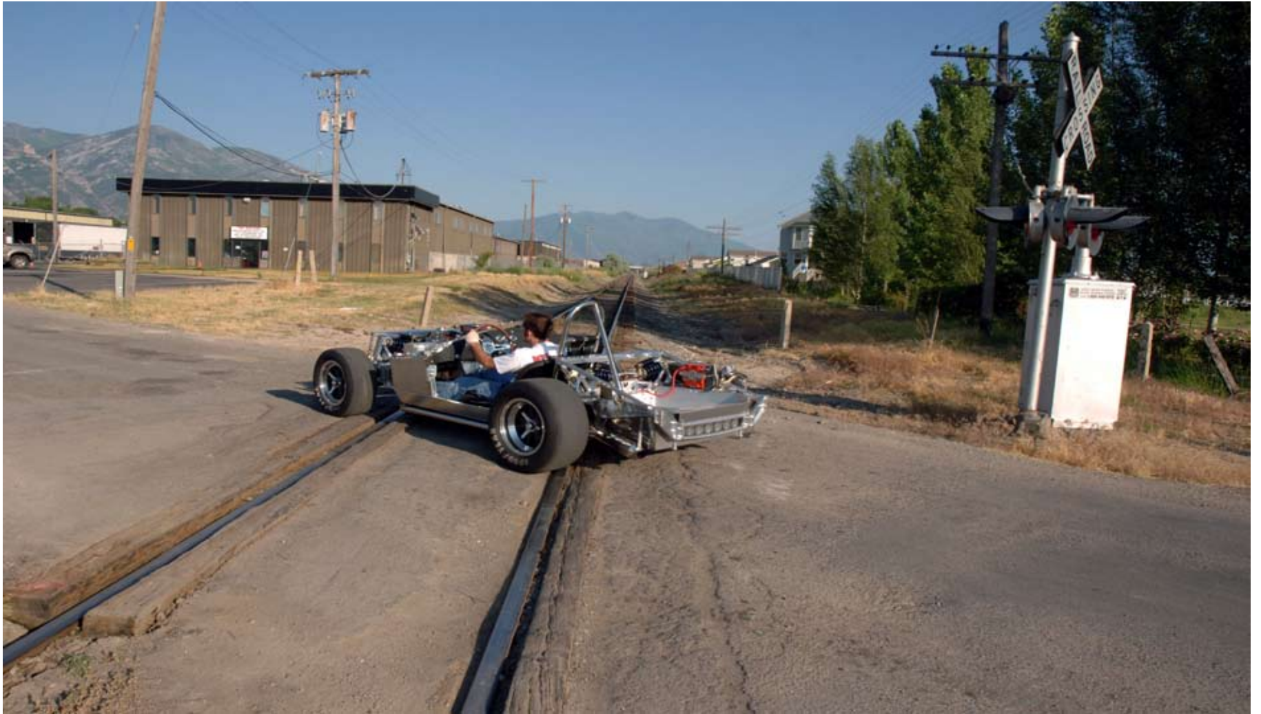
We tested the chassis at speed over railroad tracks to make sure everything was working properly under severe road conditions.
