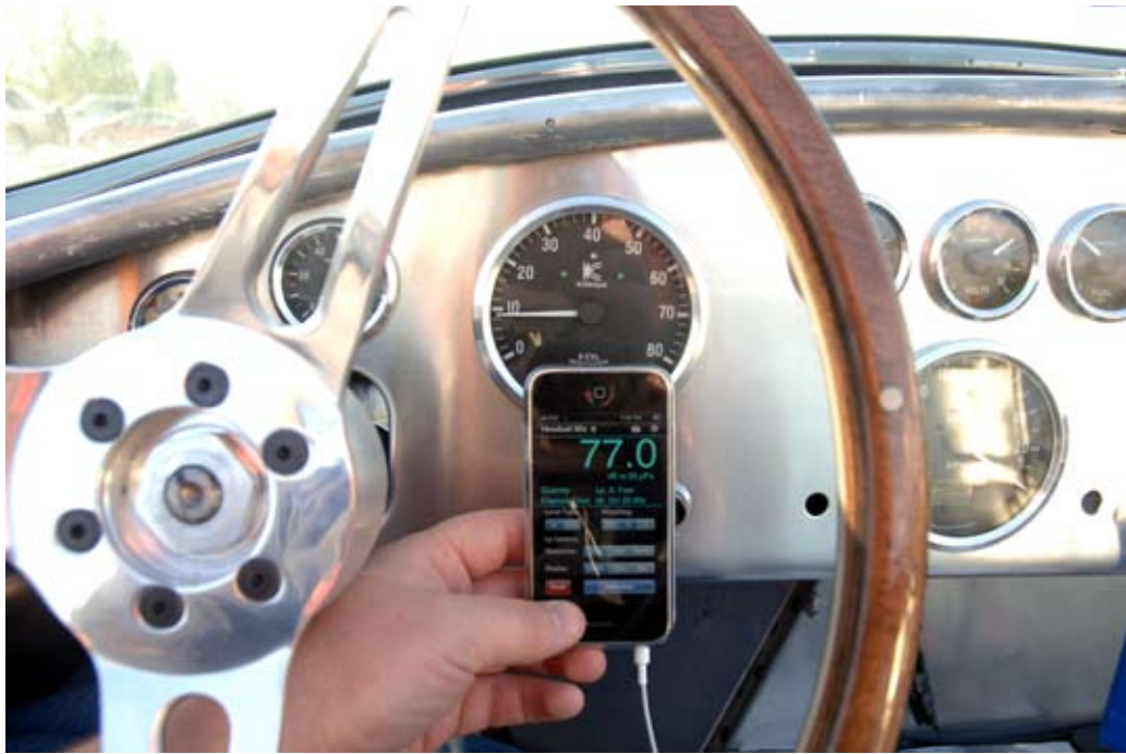
Larry wanted his car to be a little quieter than normal, so I downloaded a decibel meter for my iPhone. Here the prototype car is at idle reading 77 dB. Notice the tachometer is at 1000 rpms.
