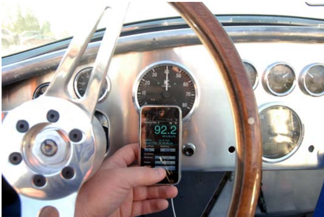
Here is the prototype car at 4000 rpms—92.2 dB.
