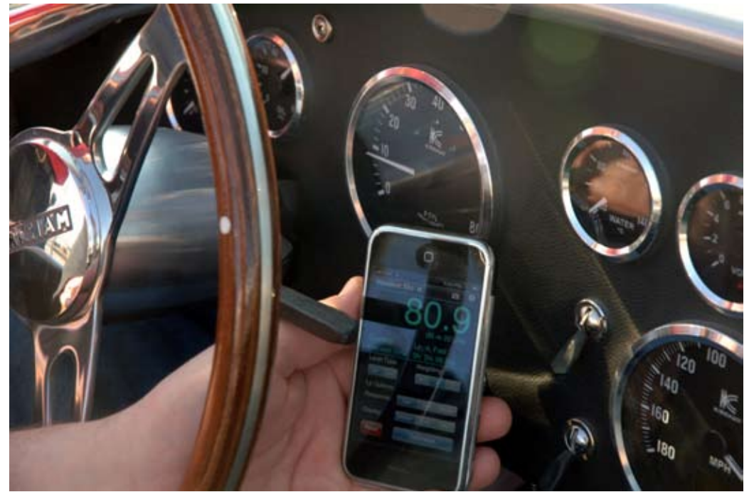
I measured one of our standard cars at 80.9 dB at 1000 rpms. Each 3 dB drop reflects a reduction in 1/2 of noise.
