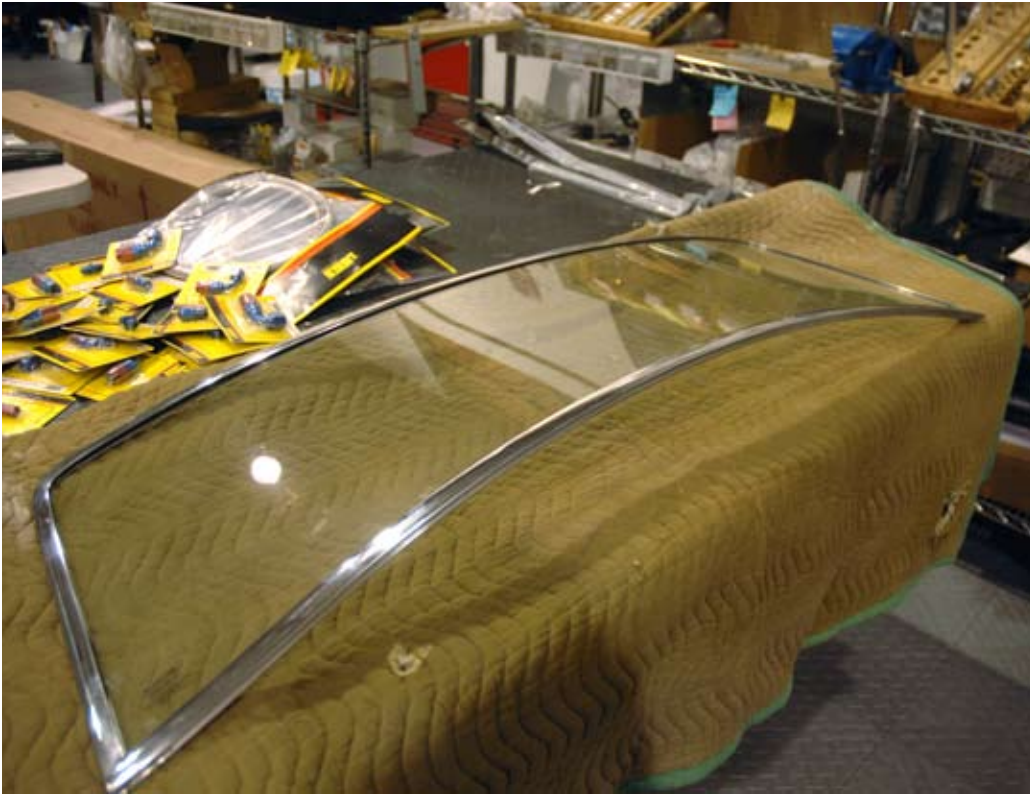
We made a special, lightweight windshield frame from aluminum. The original windshield frames are made from brass—which is four times heavier than aluminum. We removed weight everywhere we possibly could.
