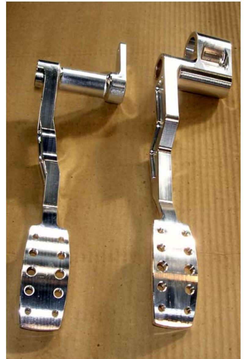
The clutch pedal is on the left and the brake pedal is on the right. The hollow cylinder at the top of the brake pedal is for the brake bias bar bearing.
