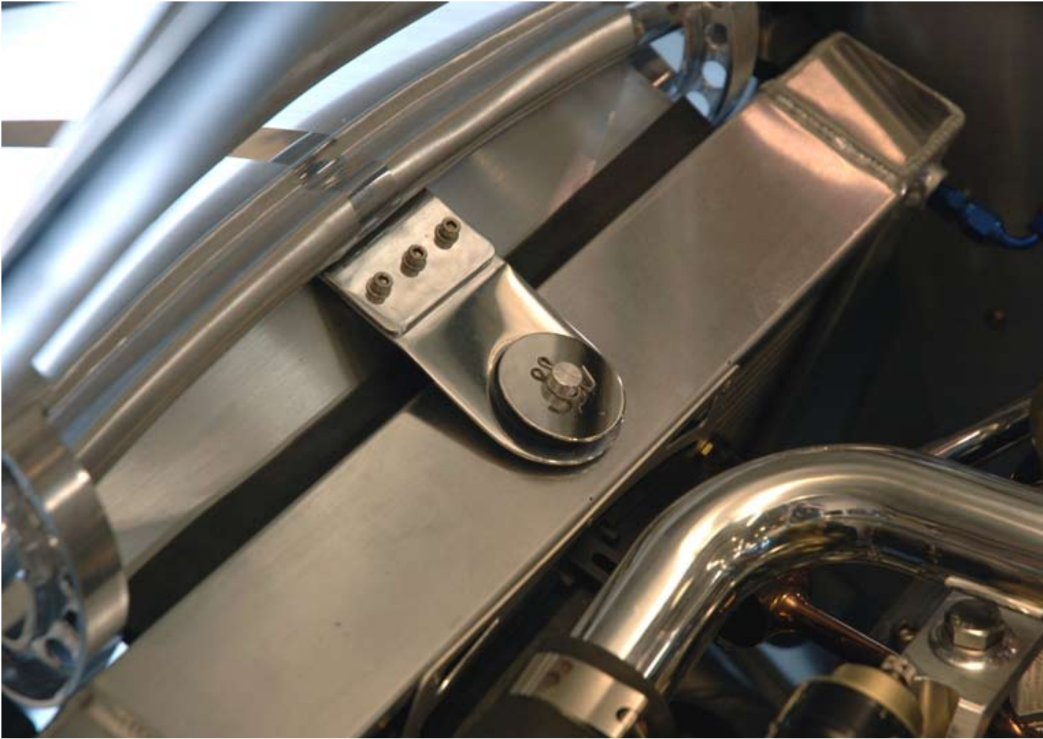
The upper radiator bracket and mounting system is identical to an original Cobra.
