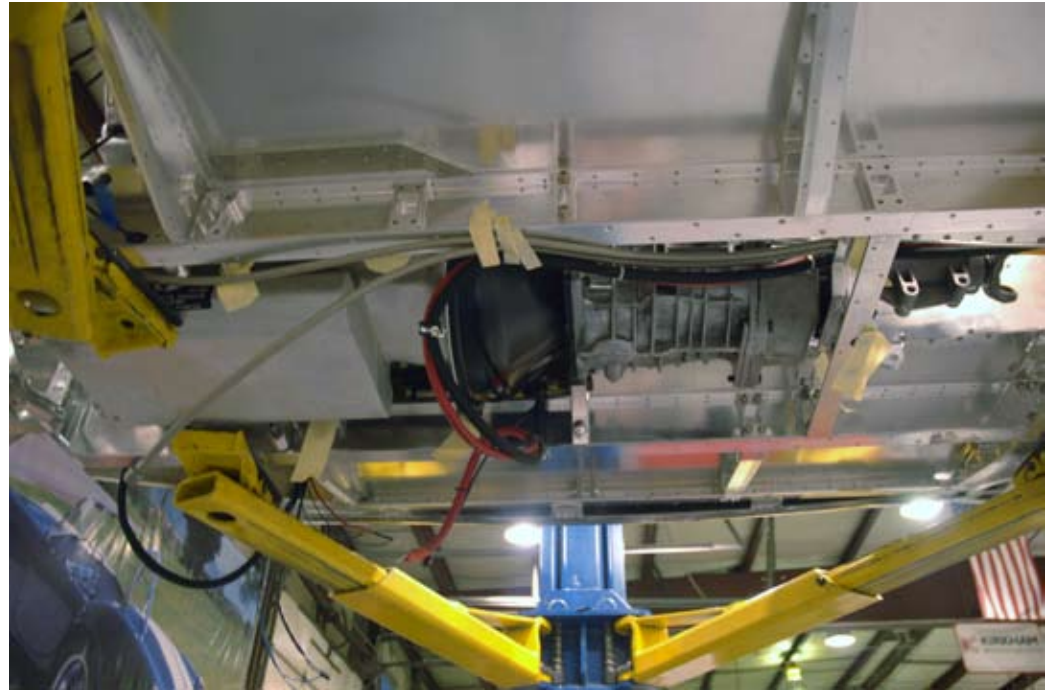
The battery cables are made from thick, 1 gauge cable. The large cable minimizes voltage drop as the car heats up.
