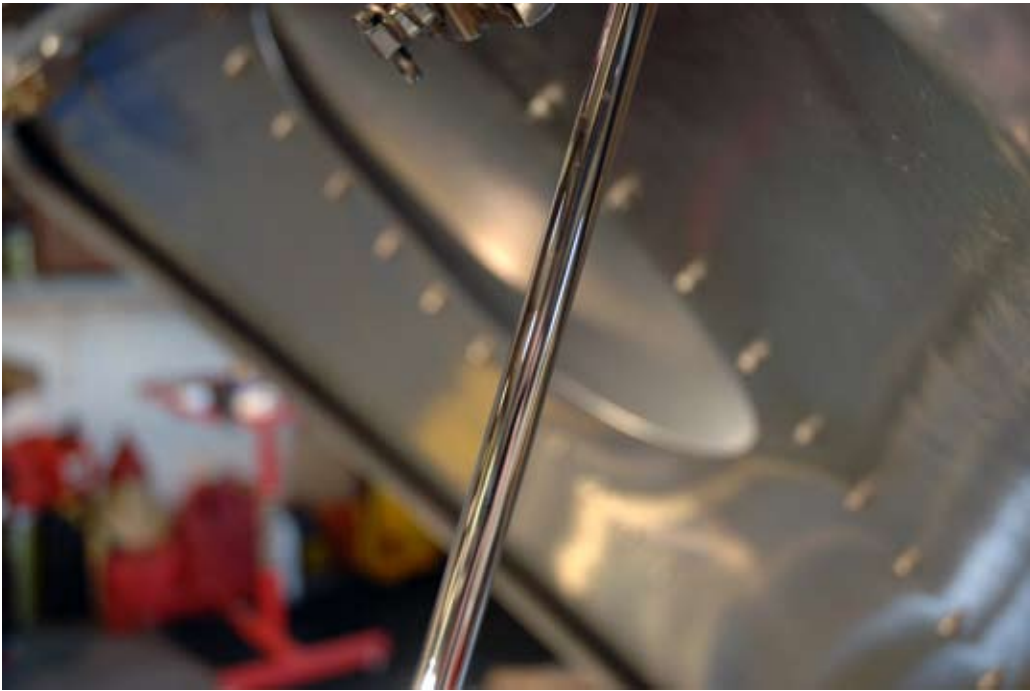
The hood prop rod was made from polished stainless steel.
