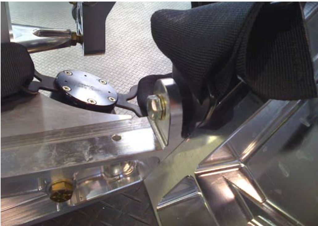
The outboard seat-belt anchor allows the seat belt to pivot on the mounting bolt so it cannot be put in a bind and torque anything in case of an accident.
