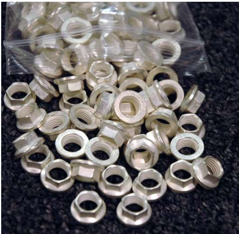
We used silver-plated stainless steel aircraft nuts. The nuts are silver plated because they are made for use on jet engines. The silver plating helps to prevent the stainless nuts from galling at the extreme temperatures encountered in jet engines. We used them because they don't rust or gall—and they look pretty sweet.
