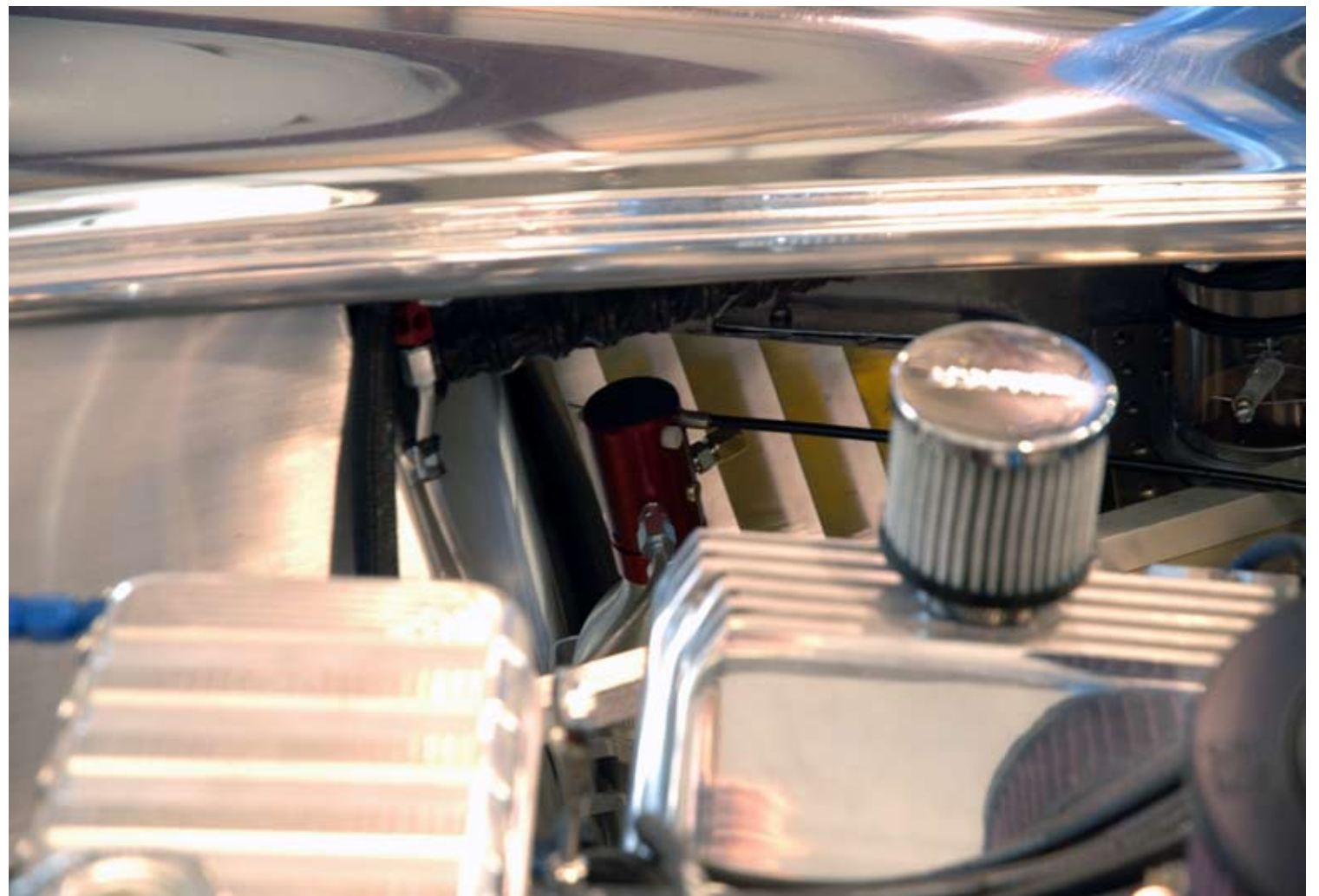
The halon fire extinguisher is mounted in the engine compartment behind the right front wheel.
