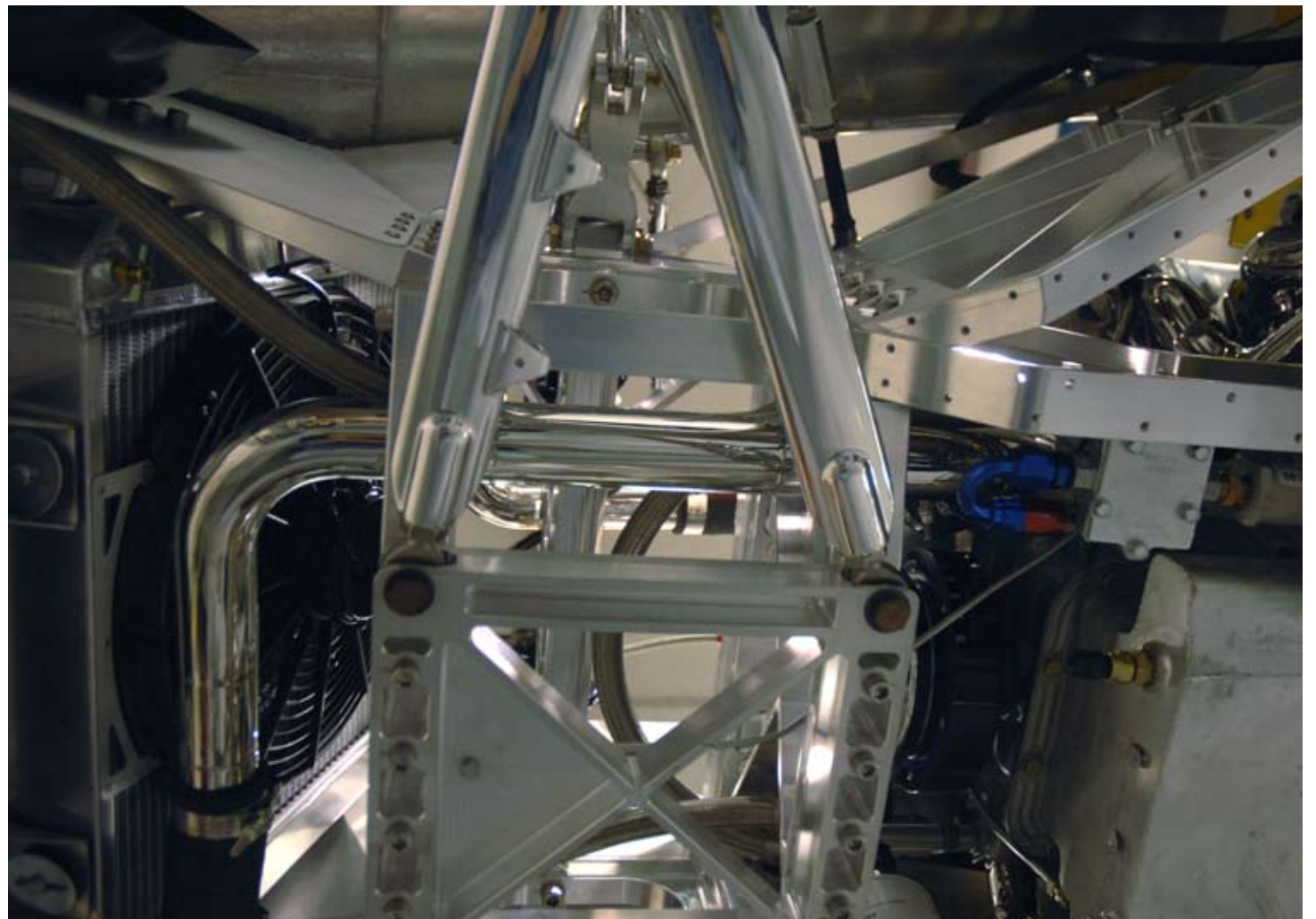
We custom made the lower radiator tube from aluminum. All fittings into the water passages on the engine were made from aluminum to prevent galvanic corrosion.
