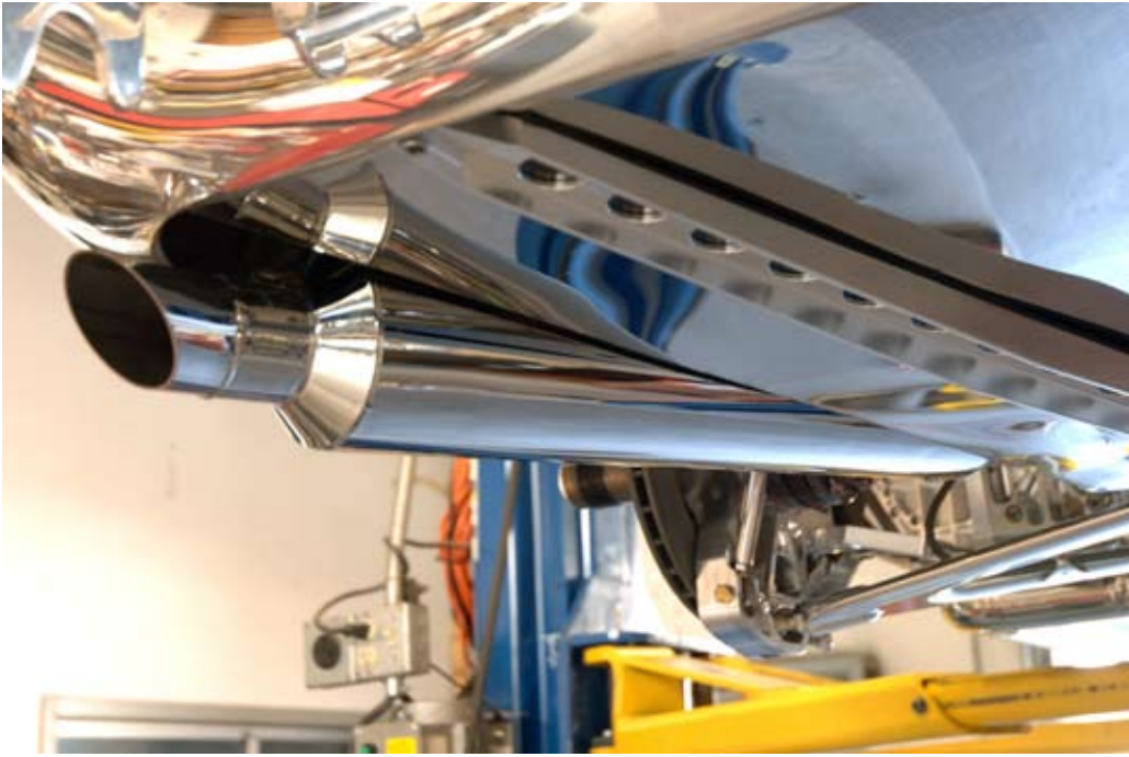
Rear exit exhaust.
