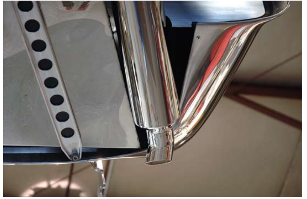
We ran the muffler as close to the gas tank as possible for minimum disruption to under-car air flow.
