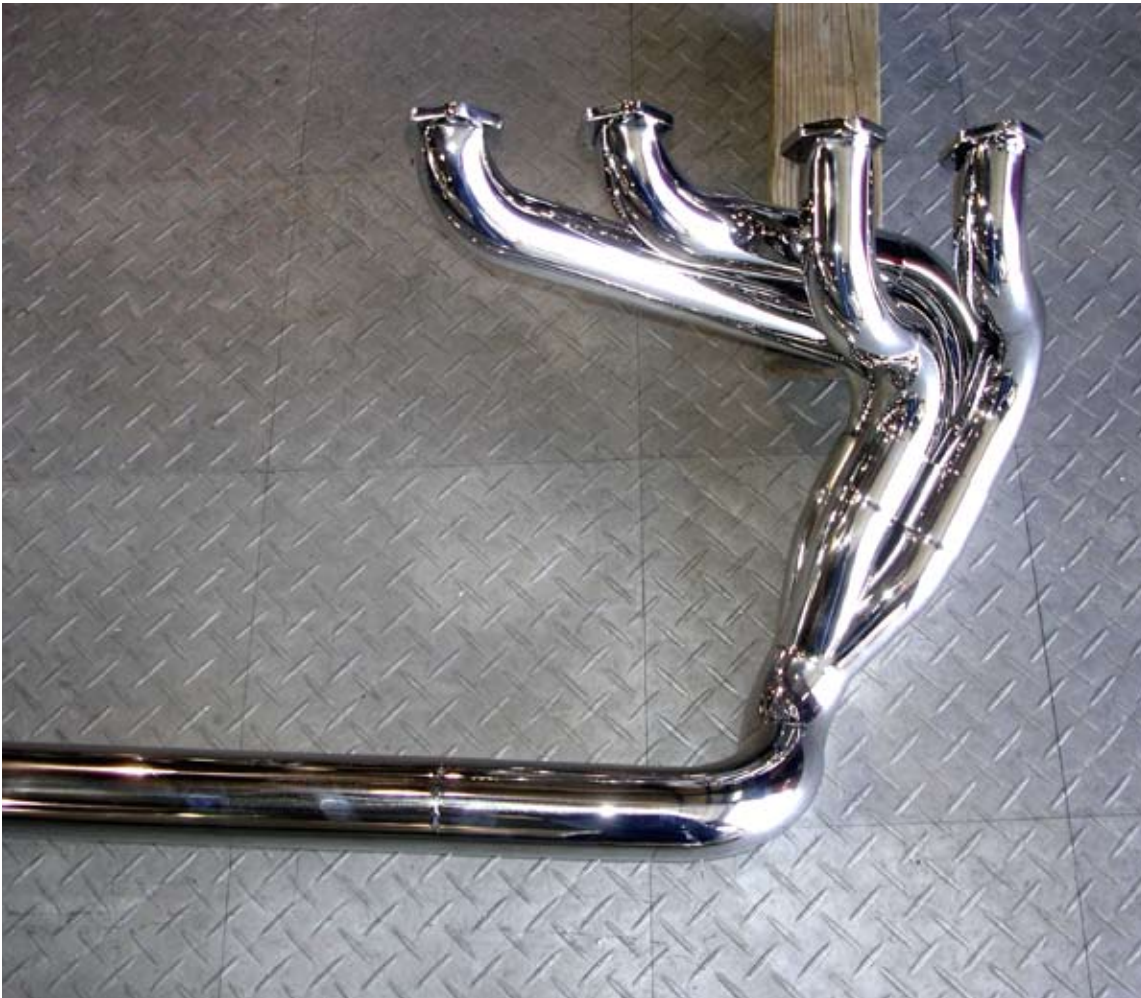
Once everything was fit, we polished the exhaust to a mirror finish. The finished exhaust was very light, compact—and beautiful.
