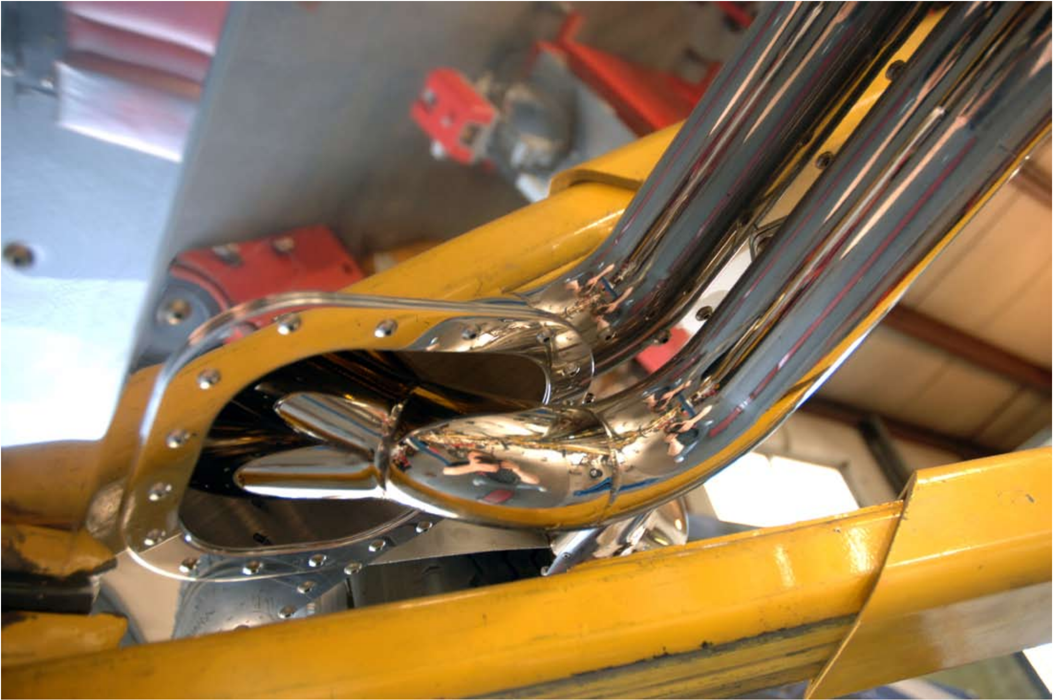
The underside of the car where the exhaust swings back up to tuck tightly against the belly pan.
