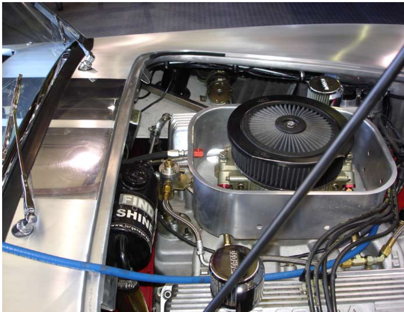
This is a picture of one of our standard cars with the engine installed. Compare with the billet car photo (above). We moved the engine back 6 inches for enhanced weight distribution.
