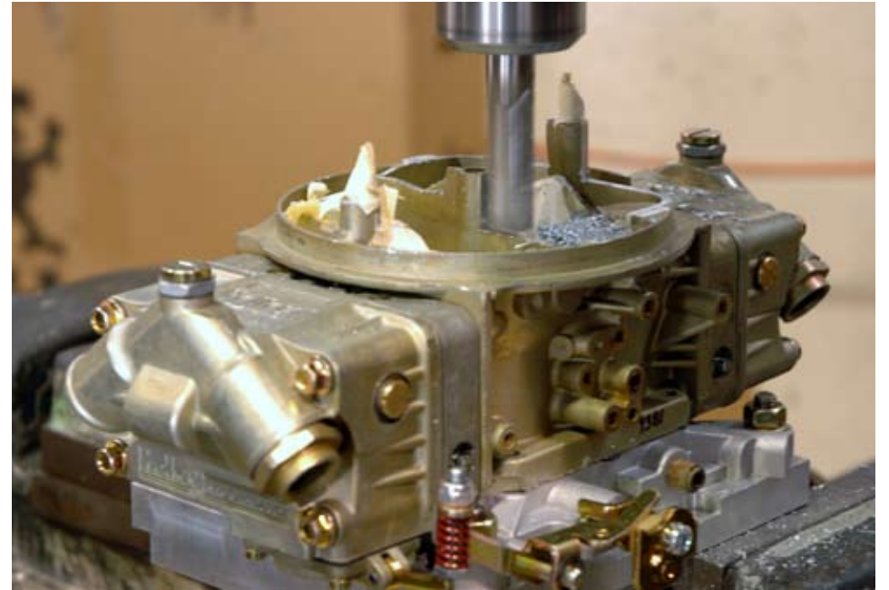
Milling off the factory air horn for greater air flow.
