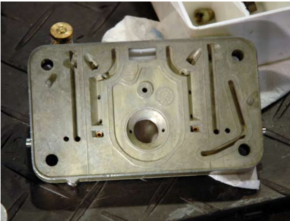
The factory fuel bleeds are too rich for the motor.
