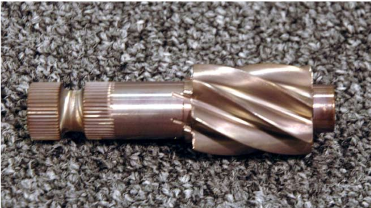
We machined the rack and pinion from Maraging 300. Maraging 300, like its name, has an ultimate tensile strength of 300,000 psi. All stainless materials are NOT the same! When Maraging 300 is hardened, it achieves a Rockwell hardness of about 52 RC—perfect for gears. Because the material is precipitation hardened—not quench hardened—we didn't have to worry about micro cracking. Maraging 300 is used to make the gears in F1 race cars. Interestingly, it is one of the only materials that can be used to make uranium centrifuges. Notice the boss on the back of the gear for a bearing—we supported the pinion on both sides to prevent any cantilever motion as the pinion was heavily loaded.
