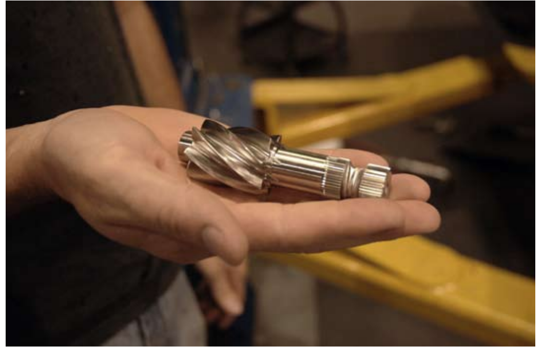
The pinion had to be extremely short so it would not hit the engine.
