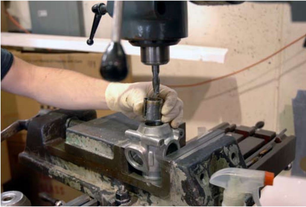
Milling the remaining part of the tube out of the housing.
