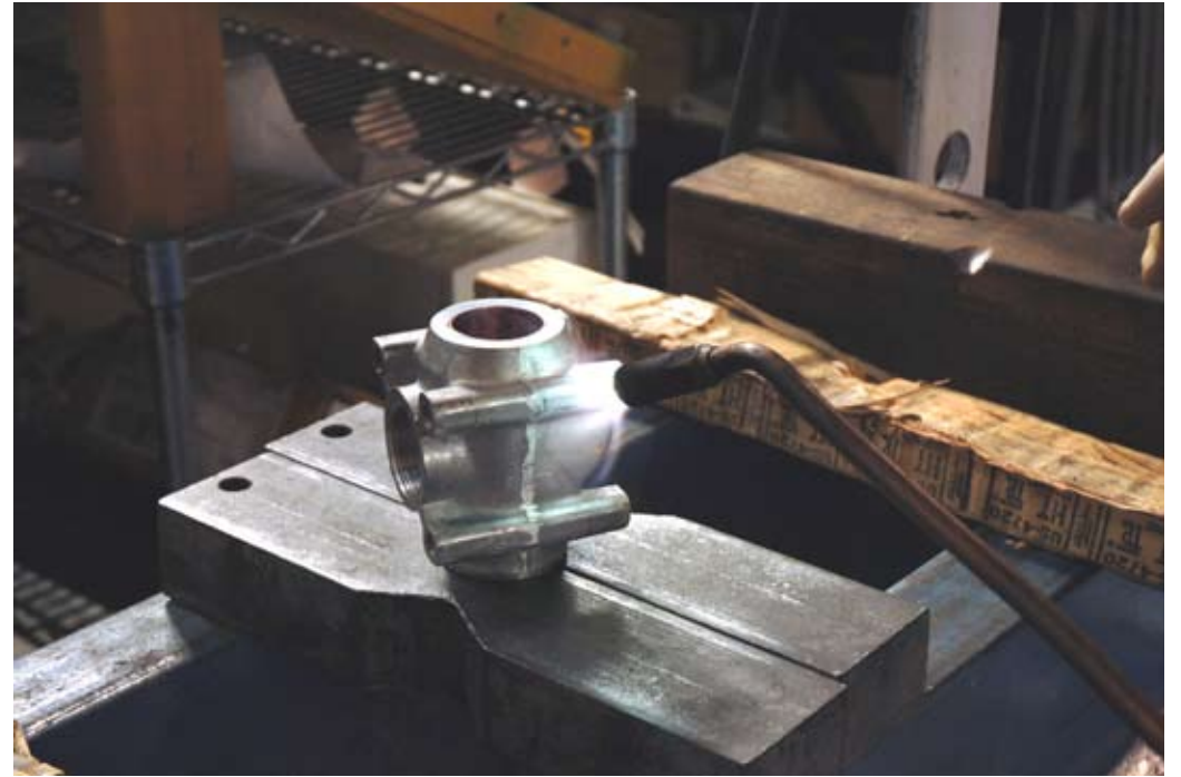
Warming up the housing to get it to expand.
