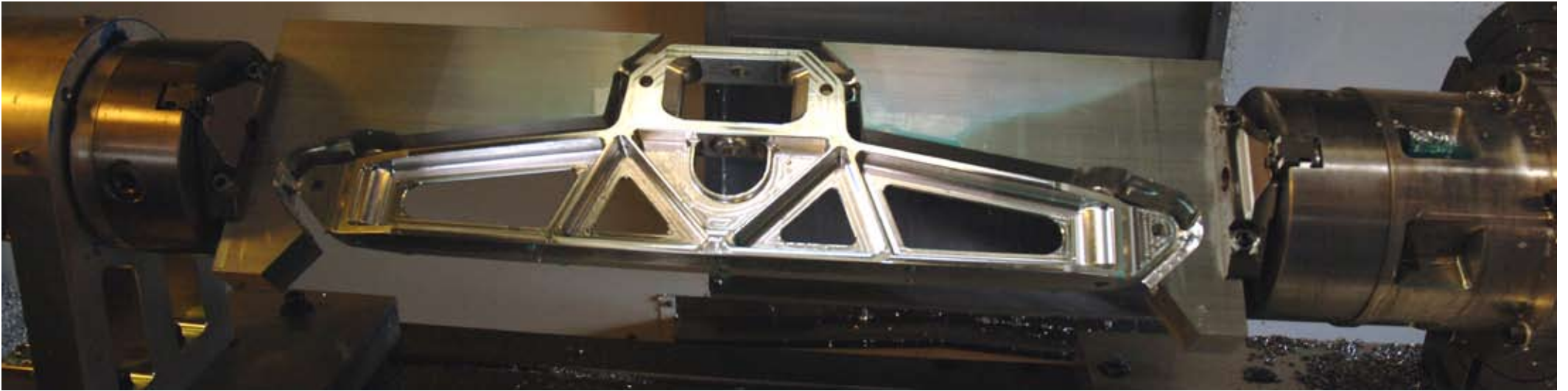
Front shock tower being machined from a solid plate of aluminum.
