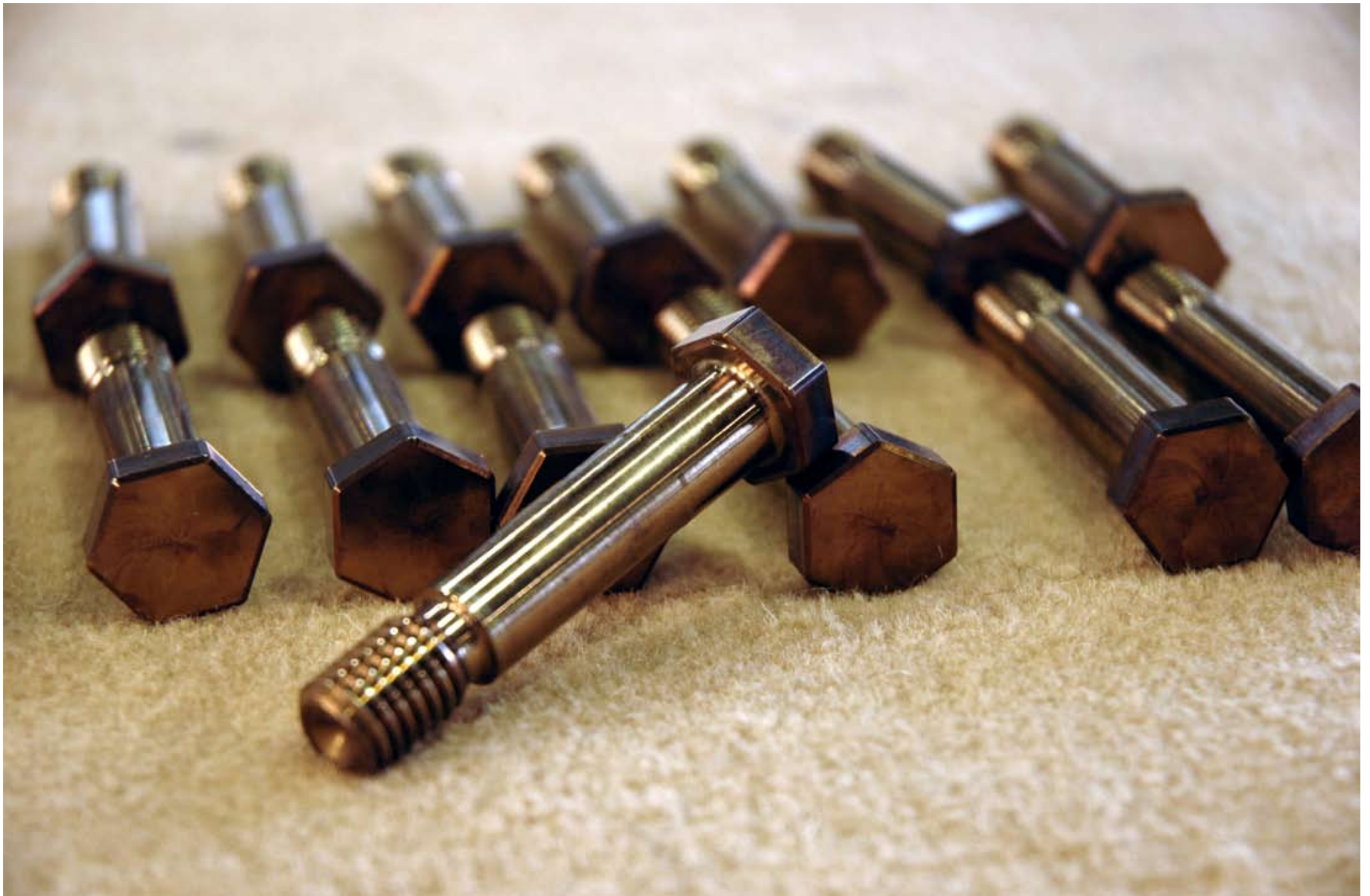
Custom control arm bolts made from 17-4 PH H900.
