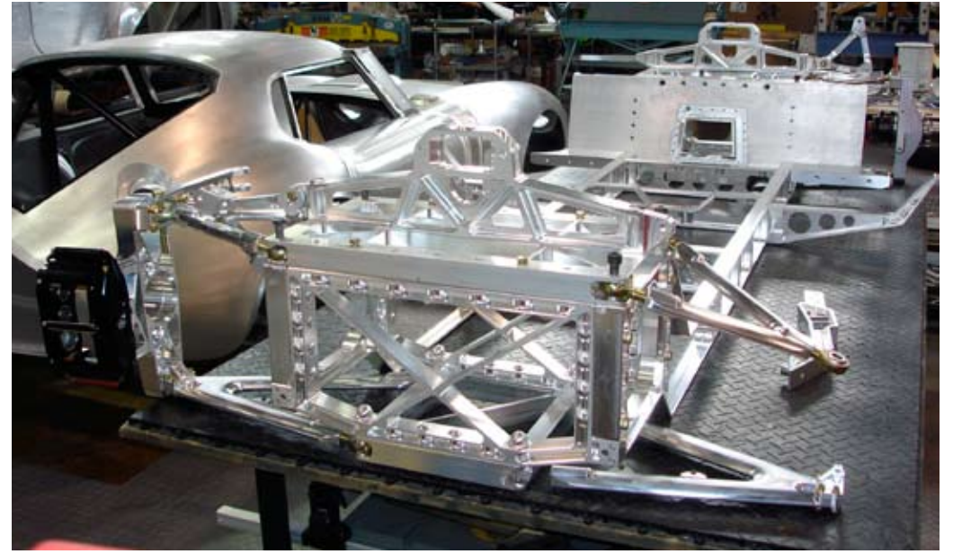
Front suspension box being assembled.
