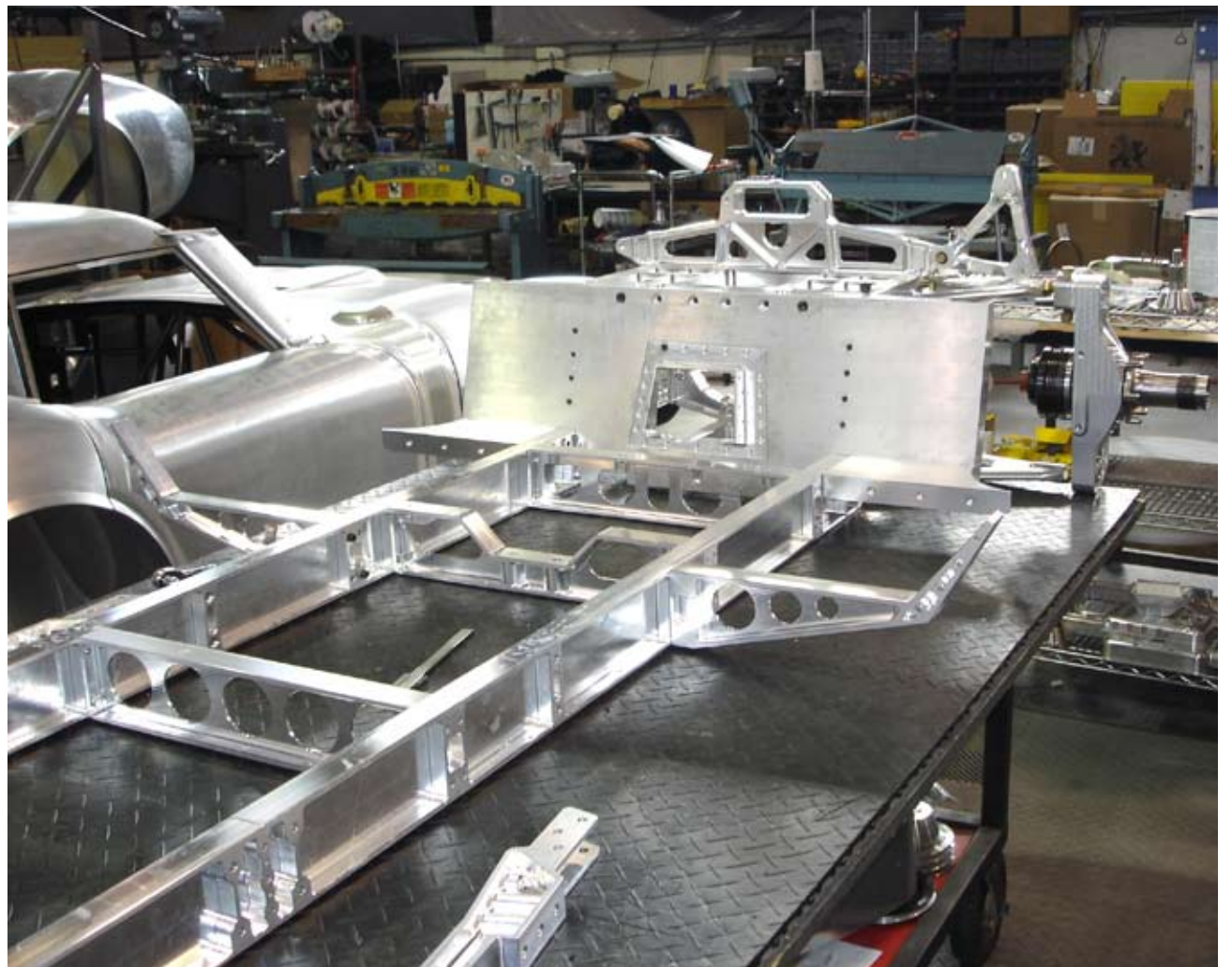
Rear suspension box assembled to the main frame rails.
