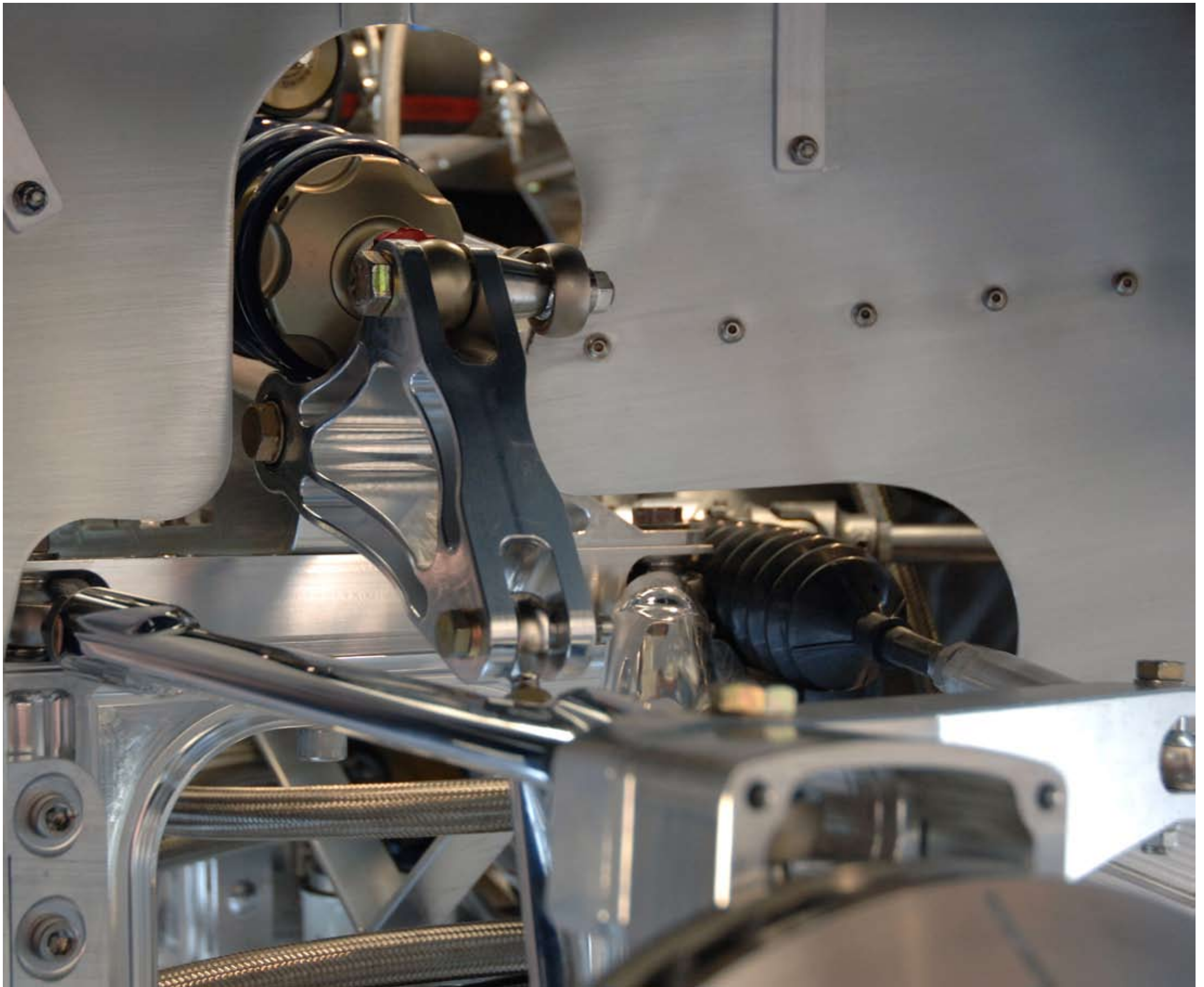
Finished front push rod and rocker assembly. The rocker pivots on roller bearings at all three points for an extremely smooth shock action. The rear rocker assembly is set up to pivot on roller bearings as well.
