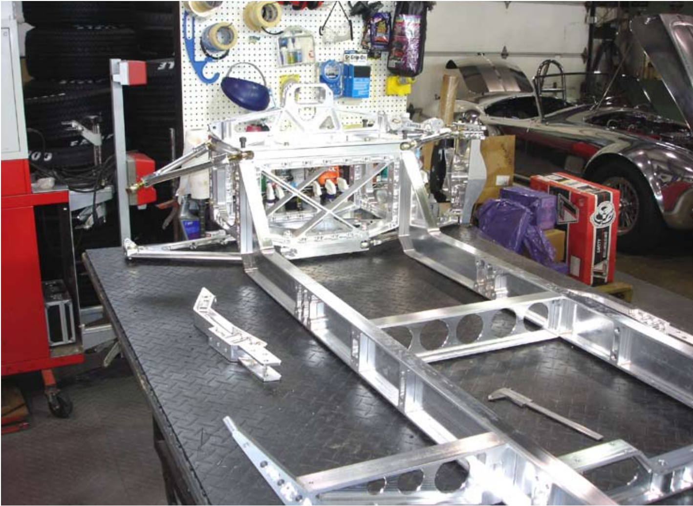
Front suspension box assembled to the main frame rails.
