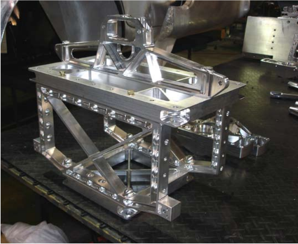
Front suspension box being assembled.
