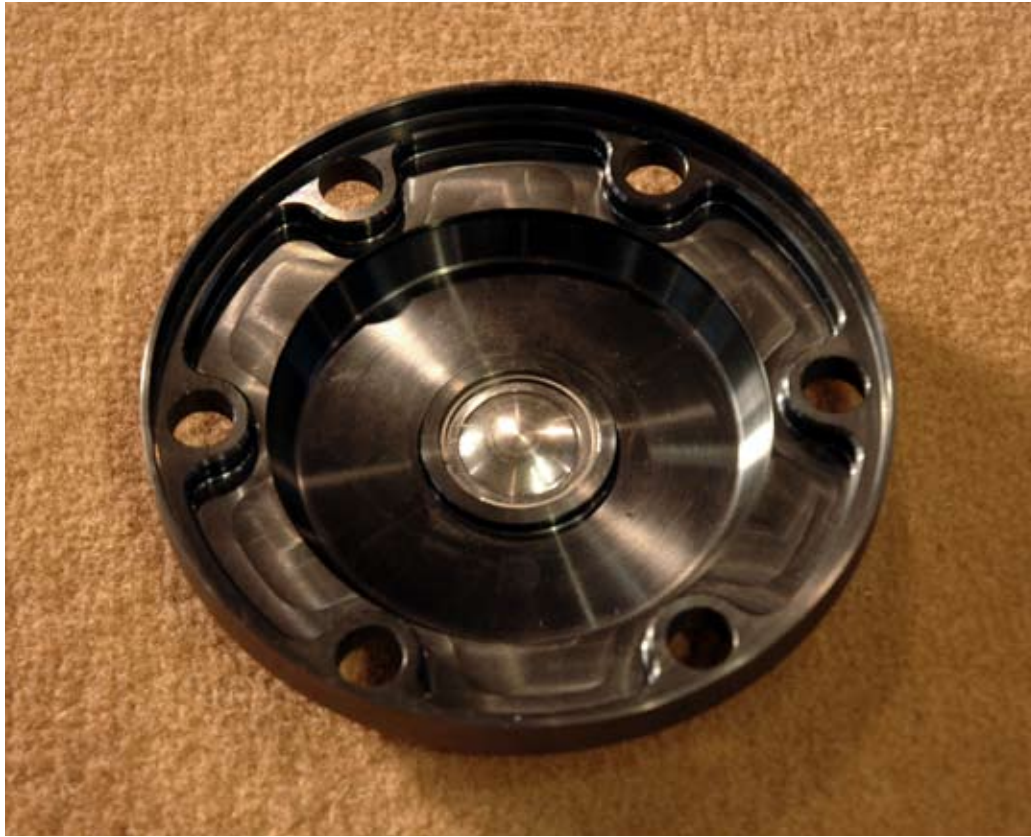
Metalore CV caps are made from the same hard material as the actual joint so they will not yield under high stress.
