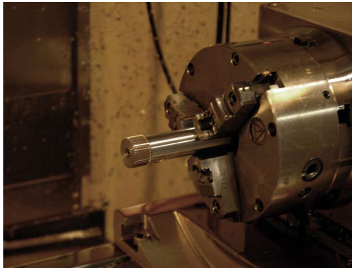
The axles were splined on one of our 4-axis mills.
