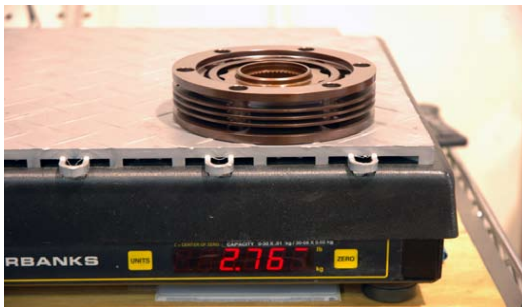
Metalore joint weighs just 2.76 pounds.
