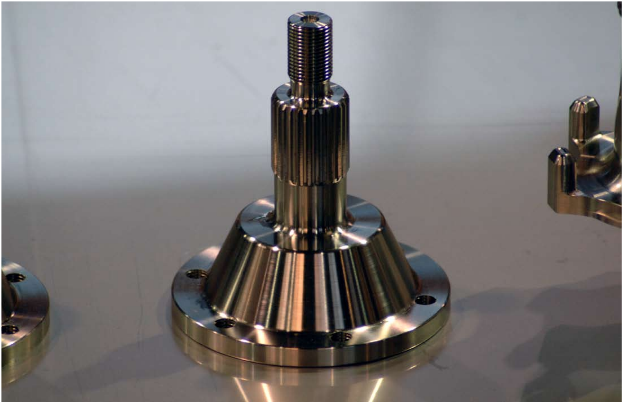
Hub side “Tulip” for the 1/2 shaft— made from 17-4 PH H900.
