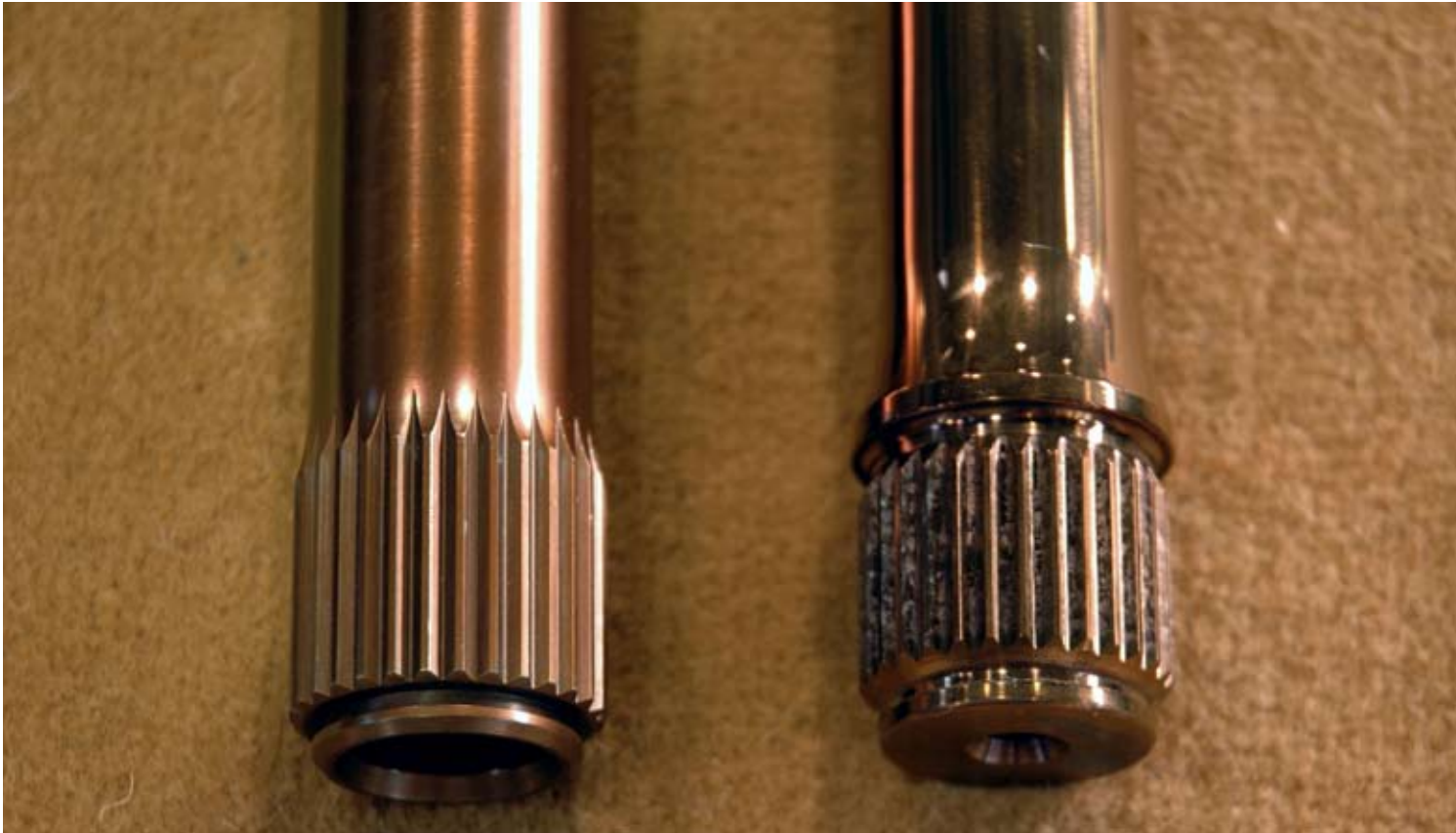
A standard Porsche axle design is on the right. We patterned our axle after the Metalore axle on the left.
