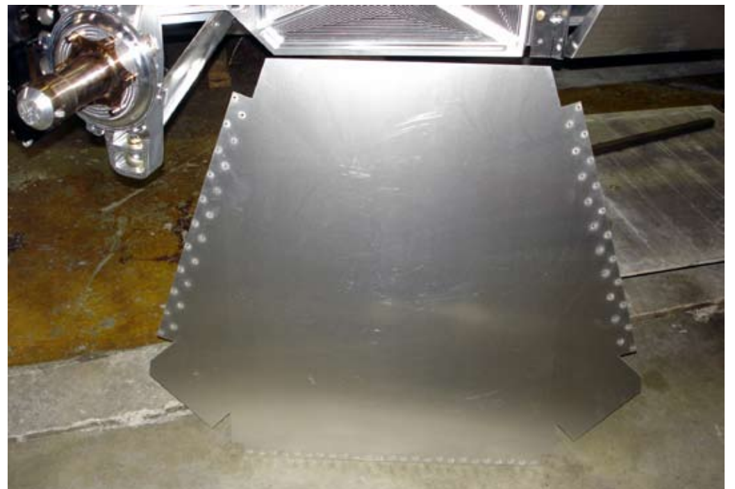
The floor of the trunk ties the entire trunk area together.
