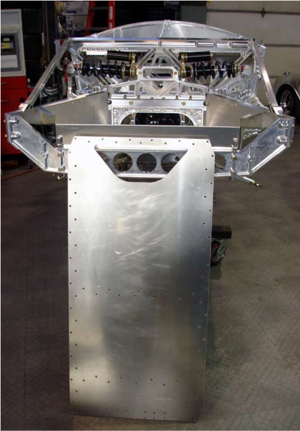
The belly pan has 87 holes that tie together 9 individual parts.
