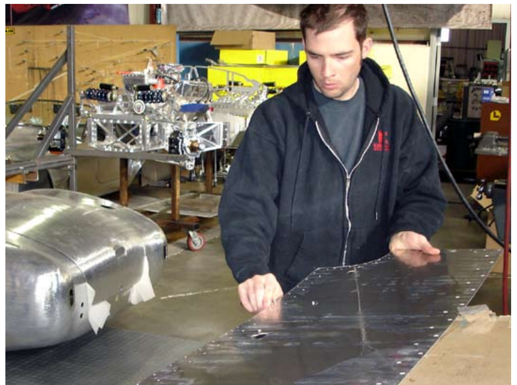
Every hole and edge in the entire car (a few thousand) was deburred on both sides—by hand if necessary.
