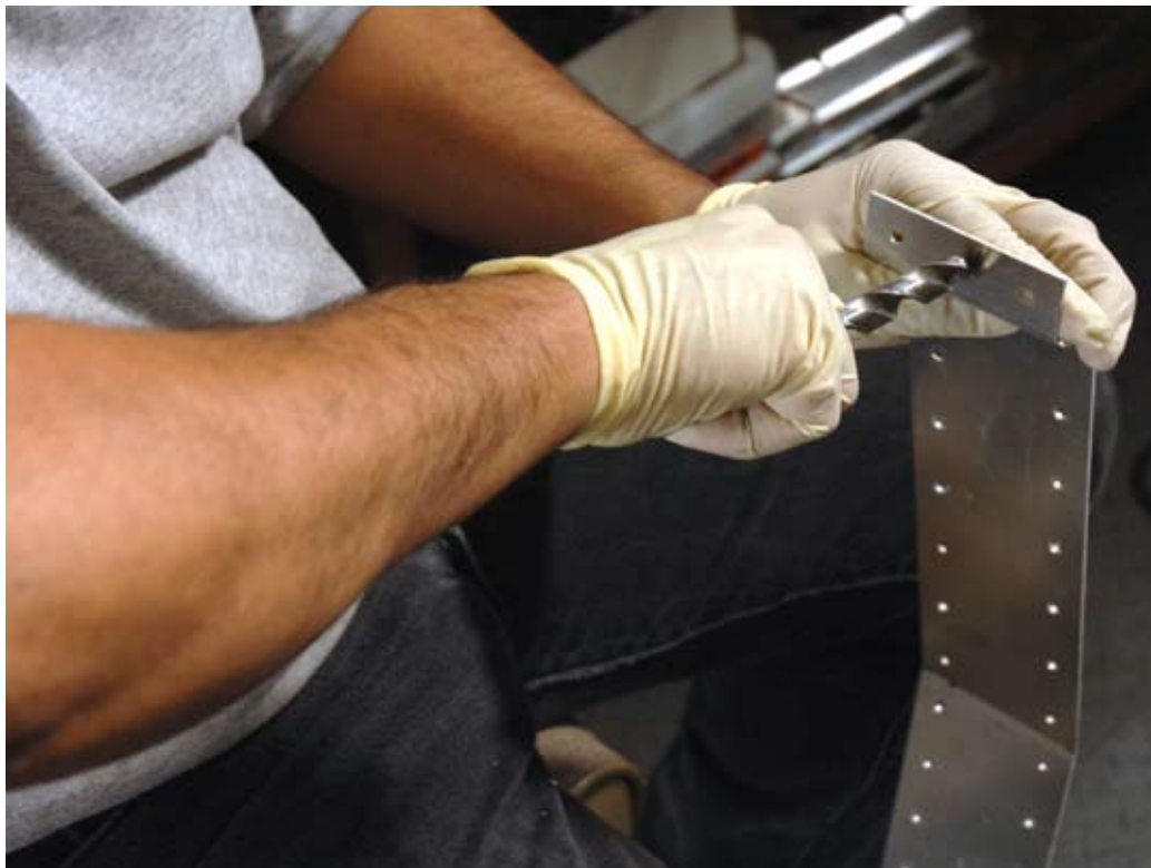
Every hole and edge in the entire car (a few thousand) was deburred on both sides—by hand if necessary.
