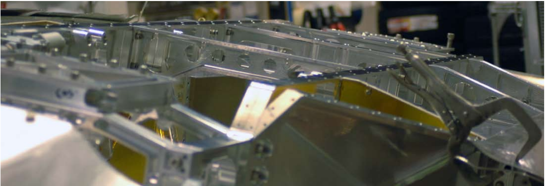
Above: A view of the final chassis during construction with no belly pans on the car. The chassis is upside-down (on a rotisserie) in this picture.
