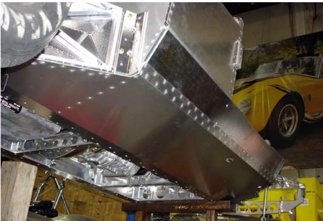
The side belly pan bolts all the way down the bottom of the rocker. The bolt holes are staggered to reduce the bending moment on the bolts, thus loading the bolts in almost pure tension and shear. The belly pans tie the rear suspension box and main frame rails all the way to the front of the footboxes.
