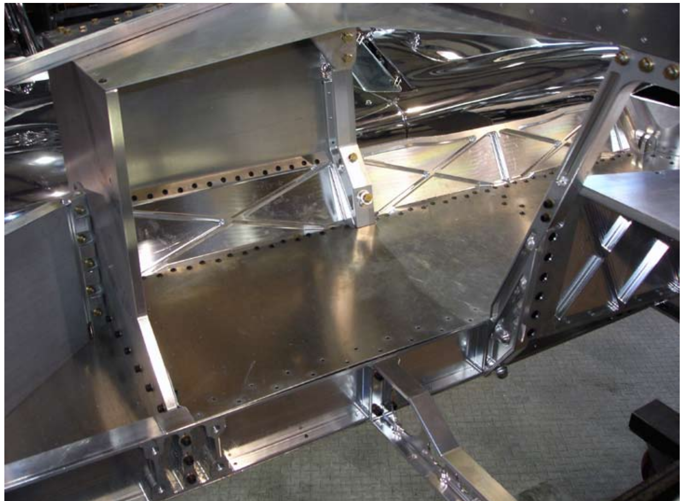
The inside of the passenger box as it was being assembled in the prototype.
