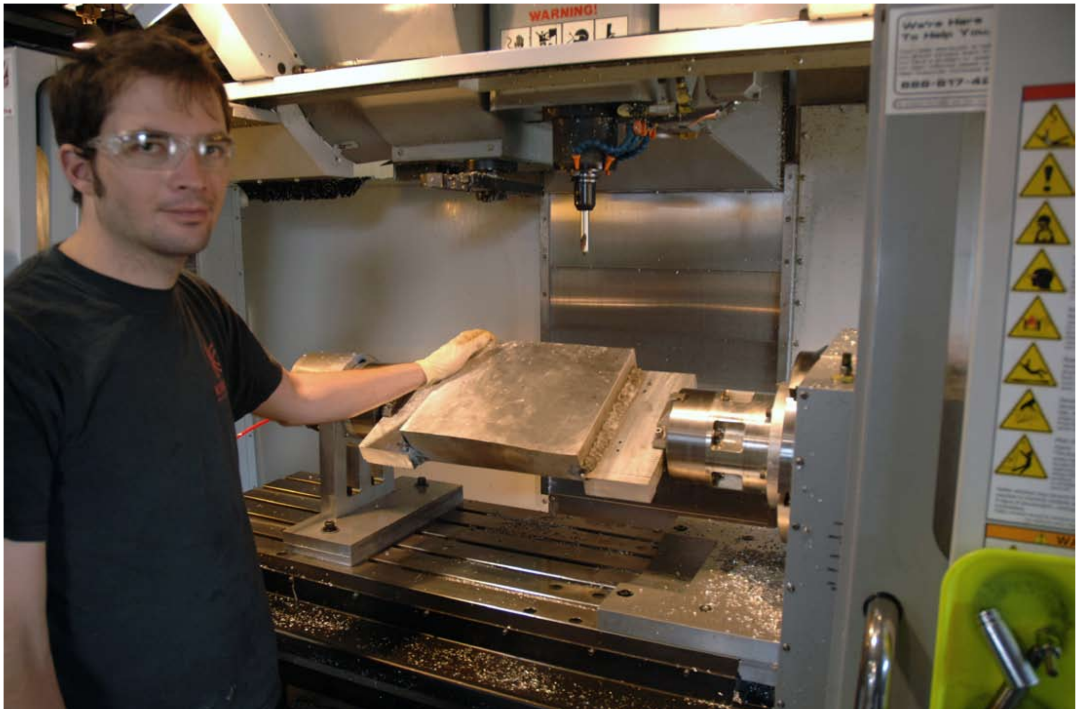
We welded some “wings” on the ends so we could hold onto the billet—they were cut off in the milling process.
