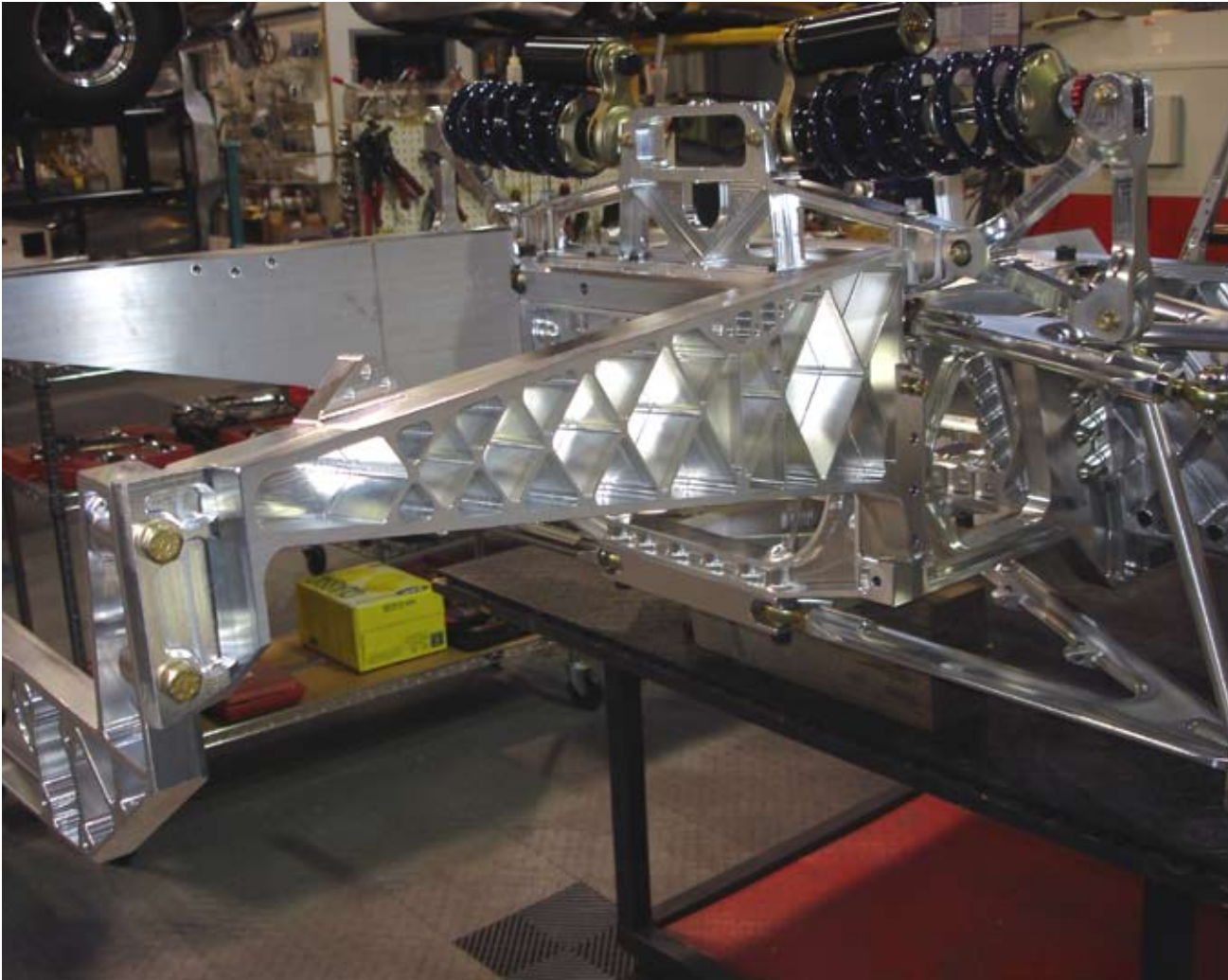
These large arms form the sides of the trunk and also must support the car when it is picked up by the jack hooks.
