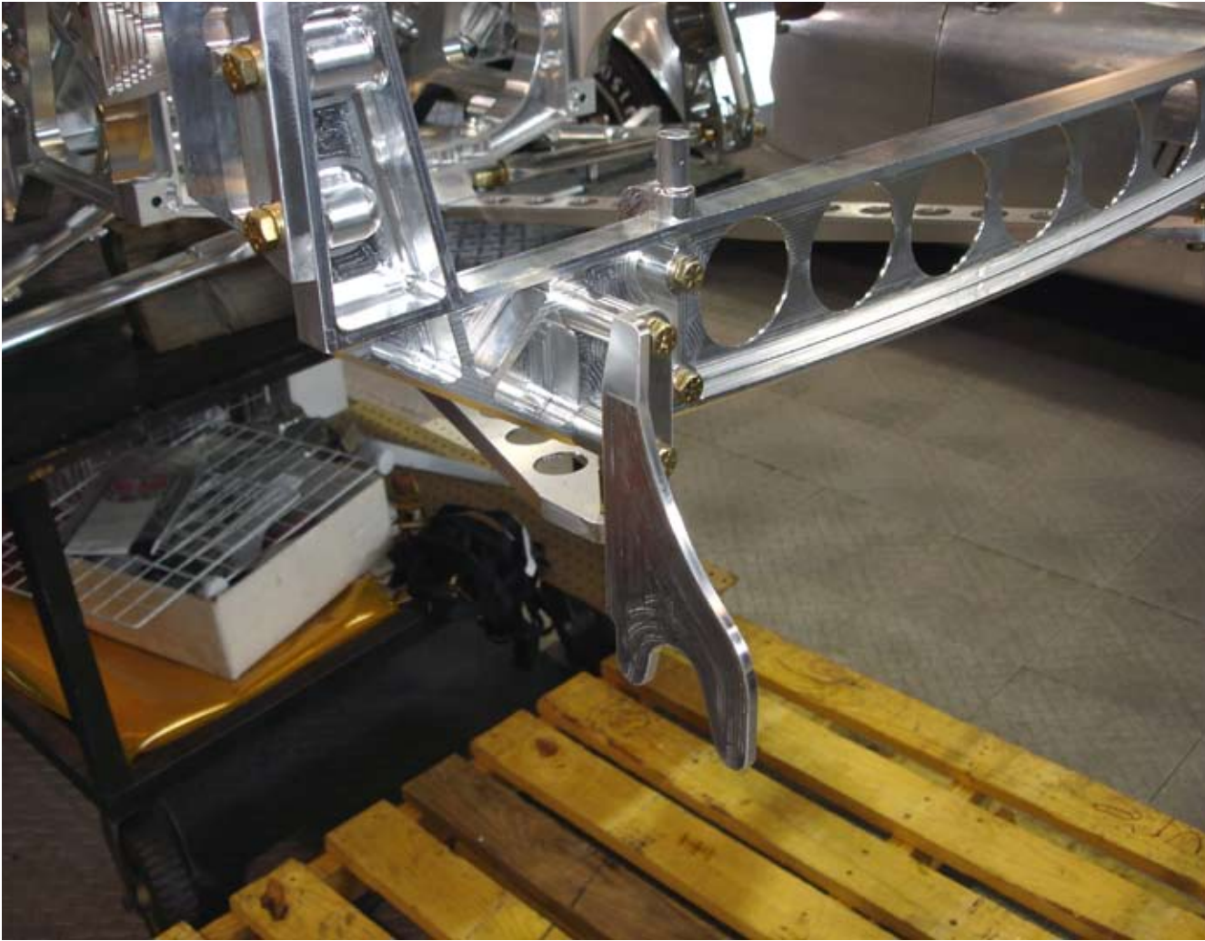
The jack hook bolts directly to the chassis.
