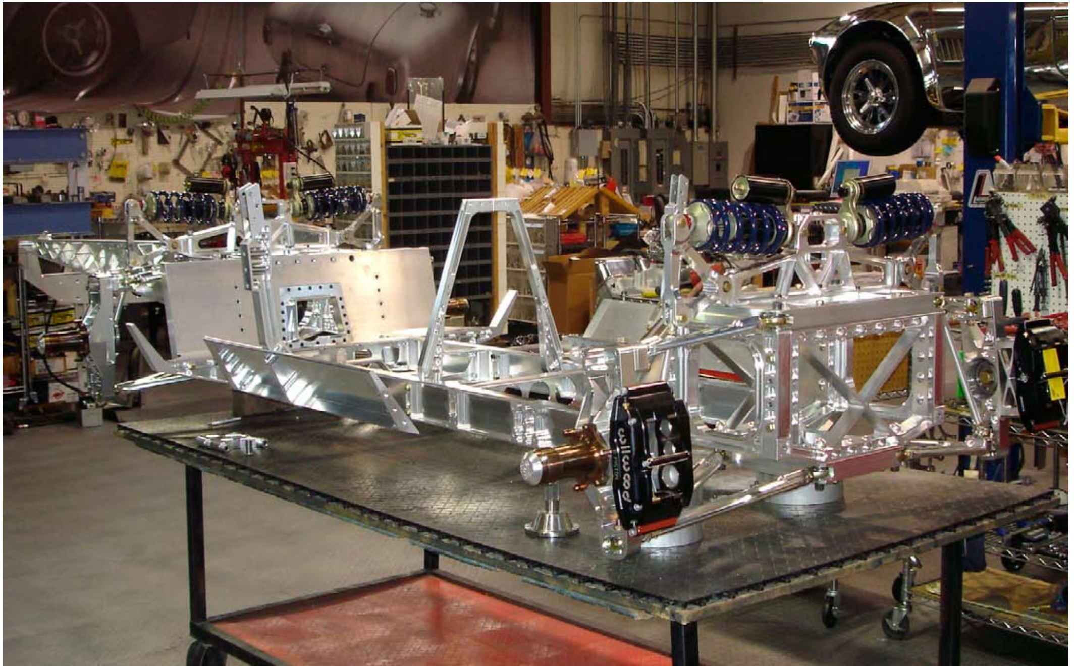
Here you can see plates under the door sills and the side cowl pillars that will support the door hinges. This shot is taken from the front—looking rearward.
