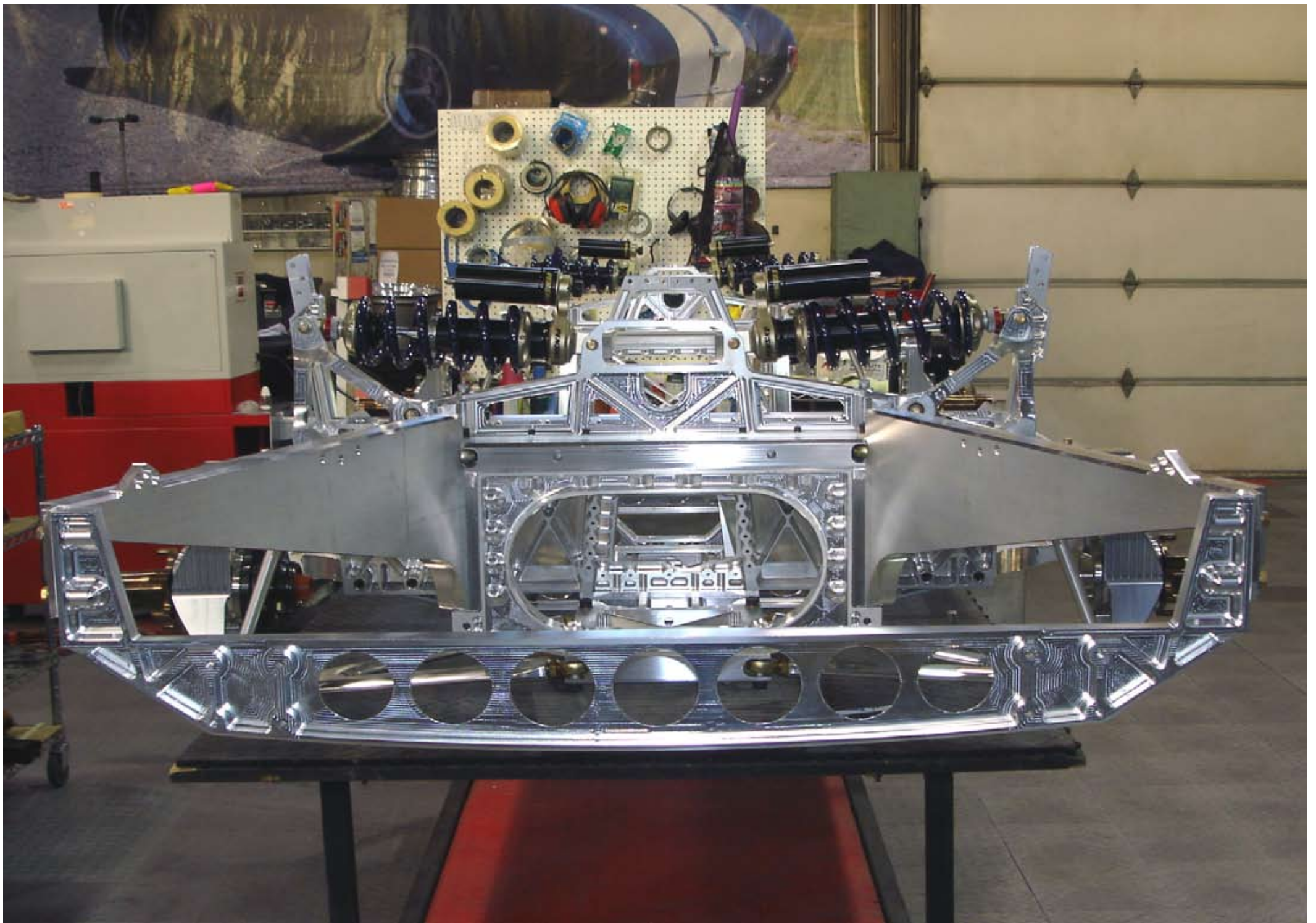
This shot is taken from the rear of the car looking forward. The side arms actually form the sides of the trunk—again, the “sheet metal” was milled directly into the parts to make them as stiff as possible.
