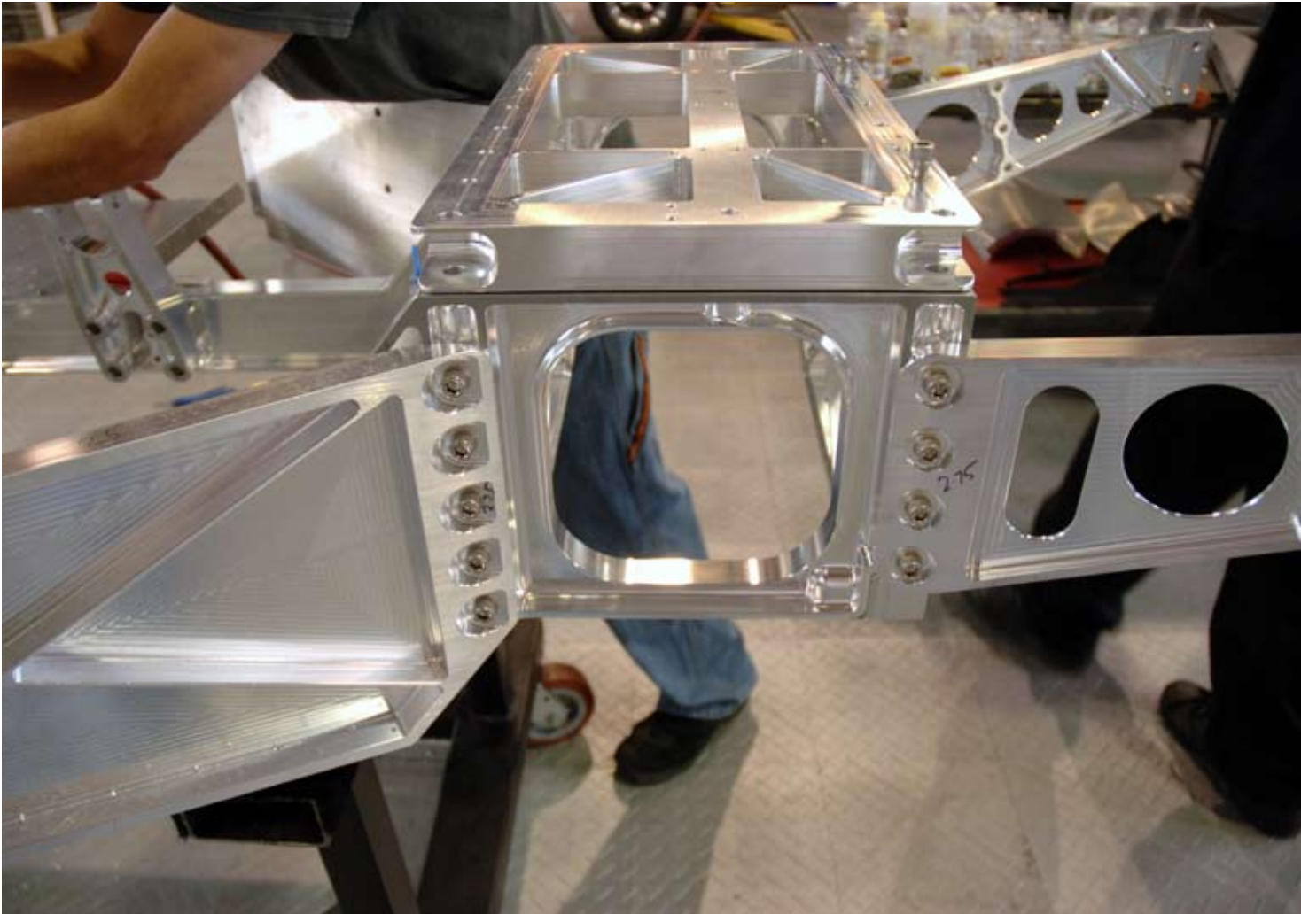
Front suspension box. The large stiffening plate in the lower left of the picture carries the loads from the front suspension to the footboxes.
