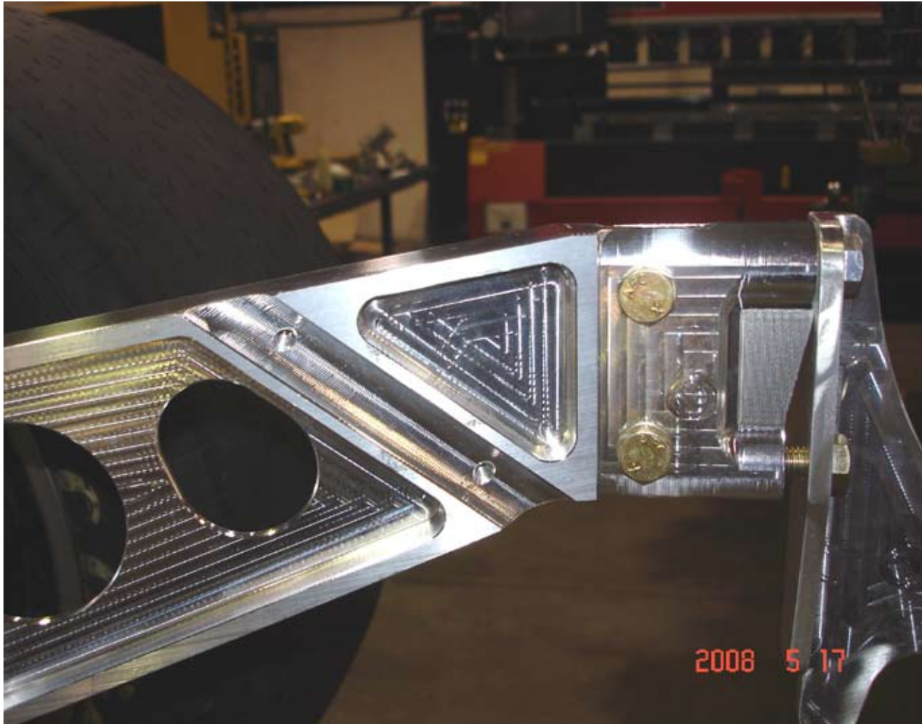
Many different angles and planes came together perfectly to make the front jack hook support.
