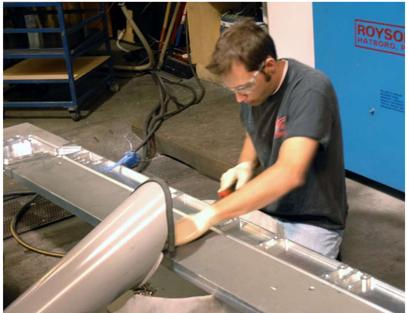
Sandwich deburring the main frame rails after the first operation. Any burrs will throw the plate out of alignment when it is put back into the fixture for the remaining operations—causing significant error over the 8 foot span of the rails.
