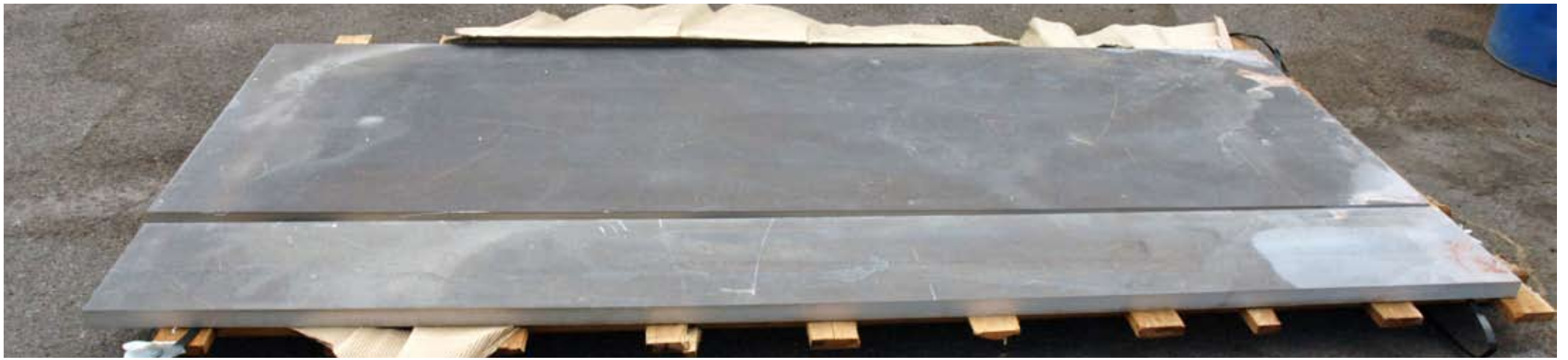
The main frame rails were first blanked out of a 1 1/2 inch x 4 foot x 12 foot plate of aluminum.
