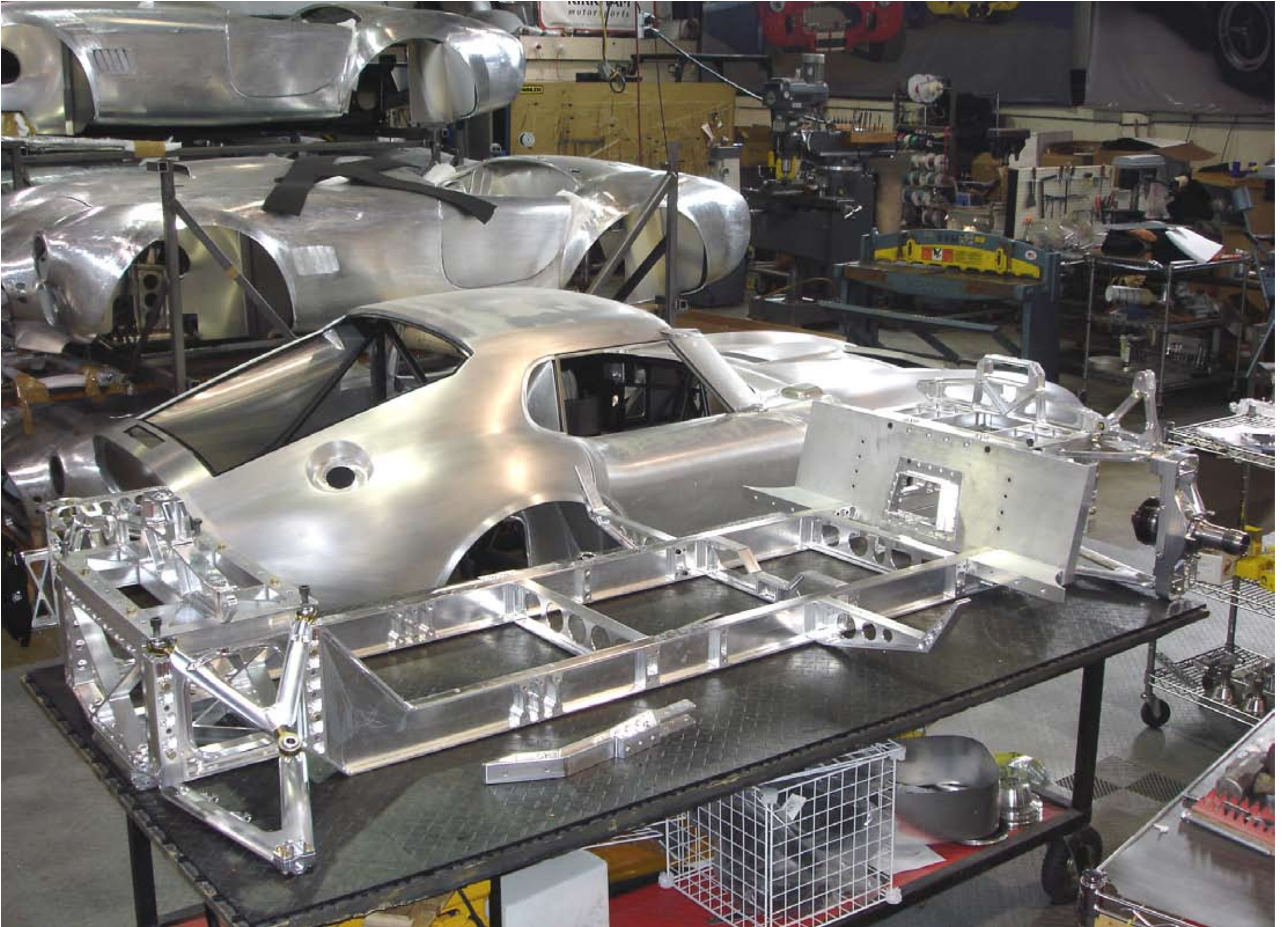
The main frame rails just as they are starting to be assembled.
